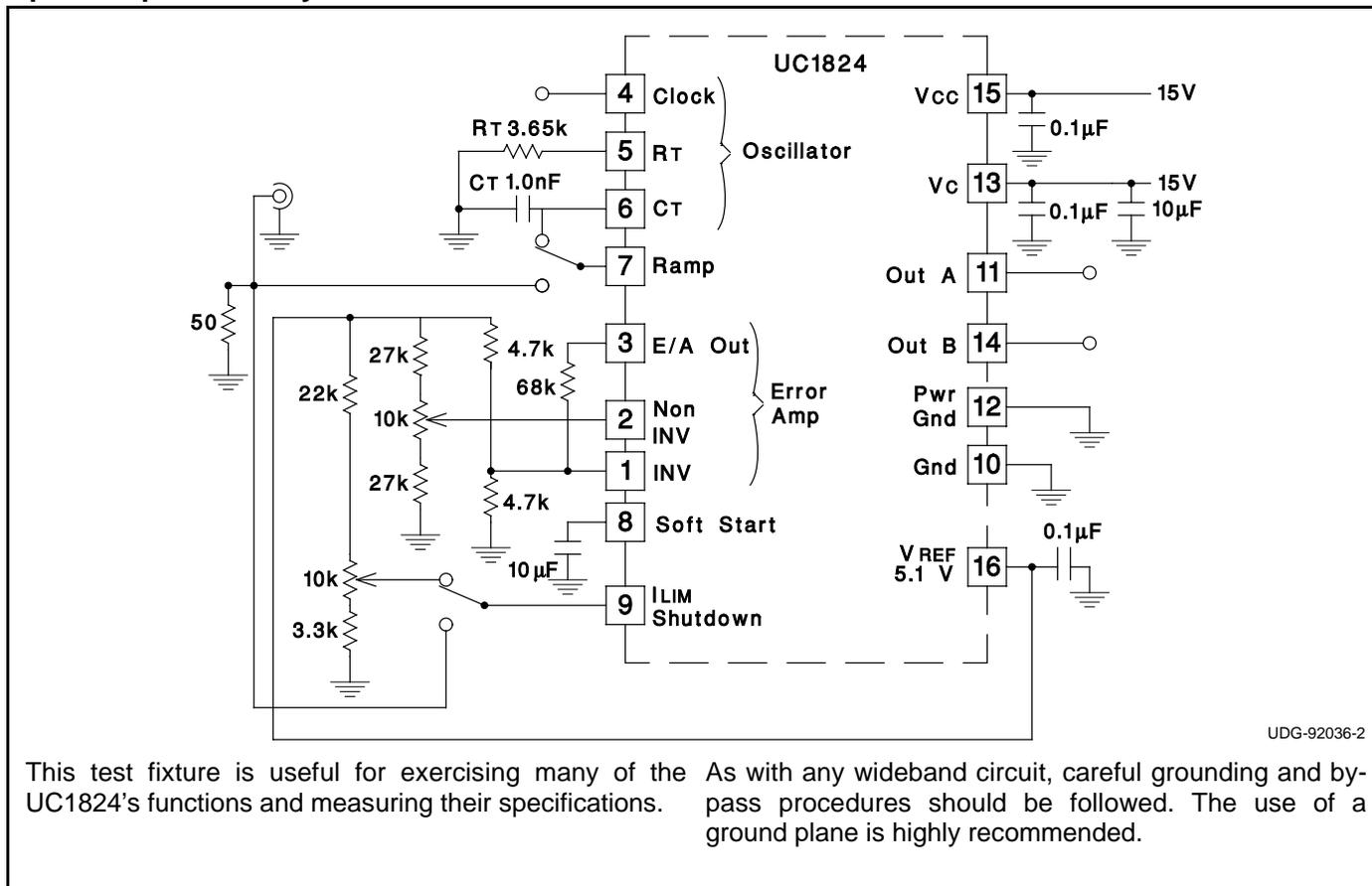
This test fixture is useful for exercising many of the UC1824's functions and measuring their specifications. As with any wideband circuit, careful grounding and bypass procedures should be followed. The use of a ground plane is highly recommended.
