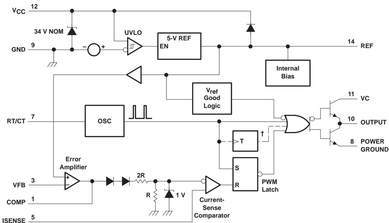
† The toggle flip-flop is present only in UC2844, UC2845, UC3844, and UC3845. Pin numbers shown are for the D Package.
