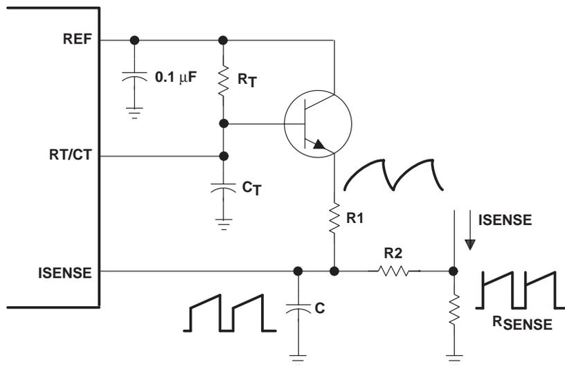
Figure 8. Slope Compensation
