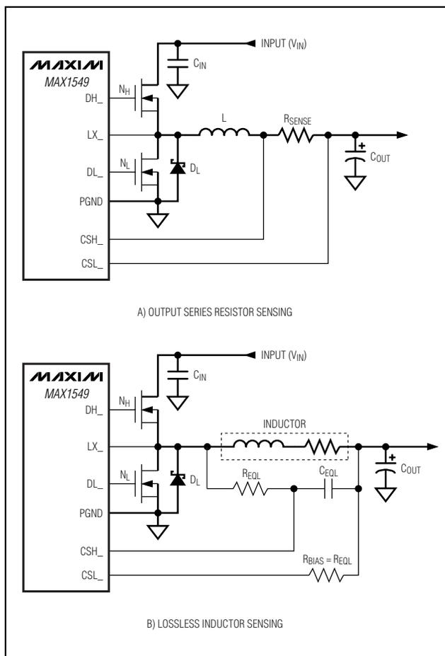
Figure 8. Current-Sense Configurations
