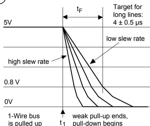
Extensive tests have shown that 1-Wire networks with lengths of up to 300m will perform best if the fall time  $t_F$  is in the range of  $4 \pm 0.5 \mu\text{s}$ . This translates into a slew rate of approximately  $1 \text{ V}/\mu\text{s}$ . This slew rate is typically achieved by selecting a PULLDOWN SLEW RATE parameter code of  $0 \times 4$  (see MODE COMMANDS). If the actual measured fall time is longer than the target value, a parameter code of  $0 \times 3$
