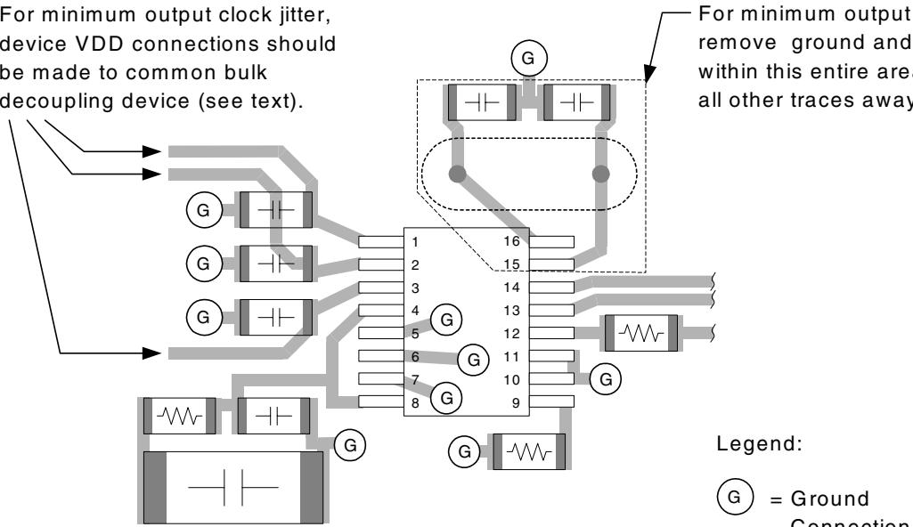
For minimum output clock jitter, remove ground and power plane within this entire area. Also route all other traces away from this area.
