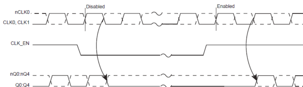
FIGURE 1. CLK_EN TIMING DIAGRAM
