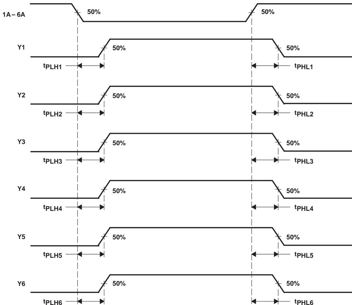
NOTE A: Output skew,  $t_{sk(o)}$ , is calculated as the greater of:
