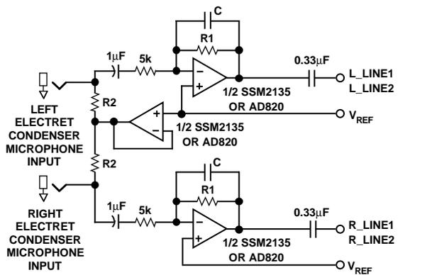
Figure 16. "Phantom-Powered" Microphone Input Circuit
