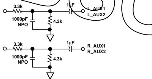
Figure 15.  $2 V_{rms}$  Line-Level Input Circuit for AUX Inputs
