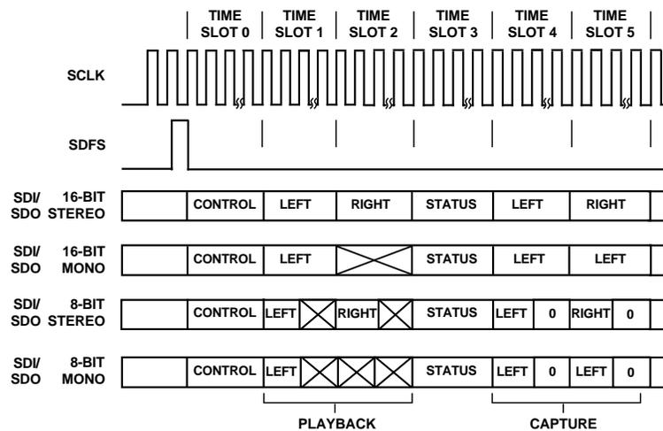
Figure 32. Serial Data Format, 1-Wire System (TSSEL = 0)
