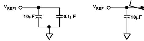
Figure 19. Voltage Reference Bypassing
