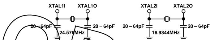
Figure 21. Crystal Connections
