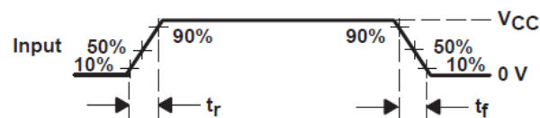
Figure 6-5. Voltage Waveforms Propagation Delay and Output Transition Times
