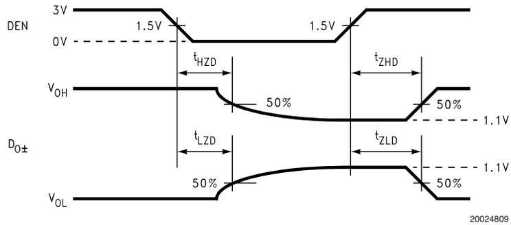
FIGURE 8. Serializer TRI-STATE Test Circuit and Timing
