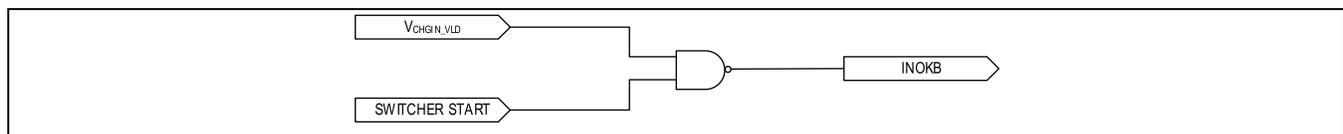
Figure 4. INOKB Signal Generation Logic
