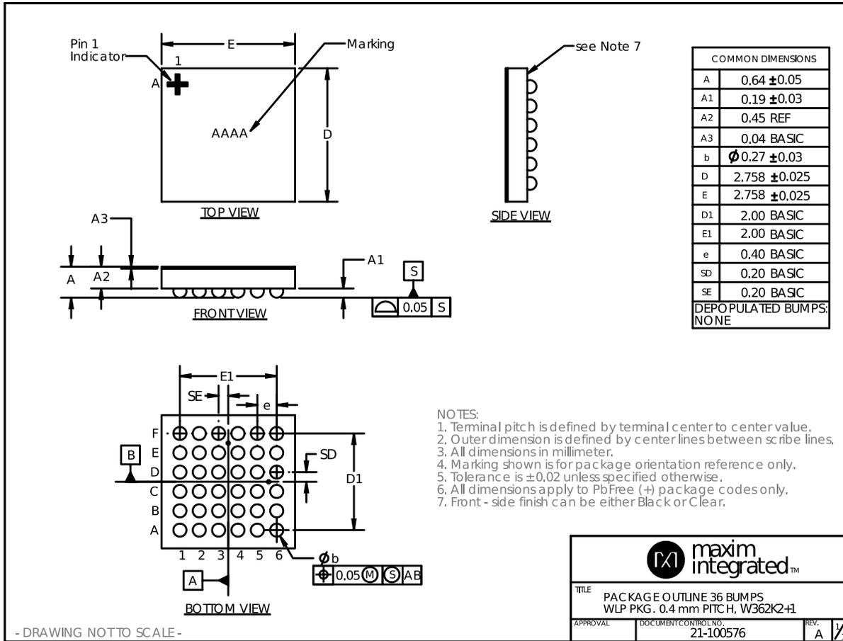
For the latest package outline information and land patterns (footprints), go to [www.maximintegrated.com/packages](http://www.maximintegrated.com/packages). Note that a "+", "#", or "-" in the package code indicates RoHS status only. Package drawings may show a different suffix character, but the drawing pertains to the package regardless of RoHS status.
