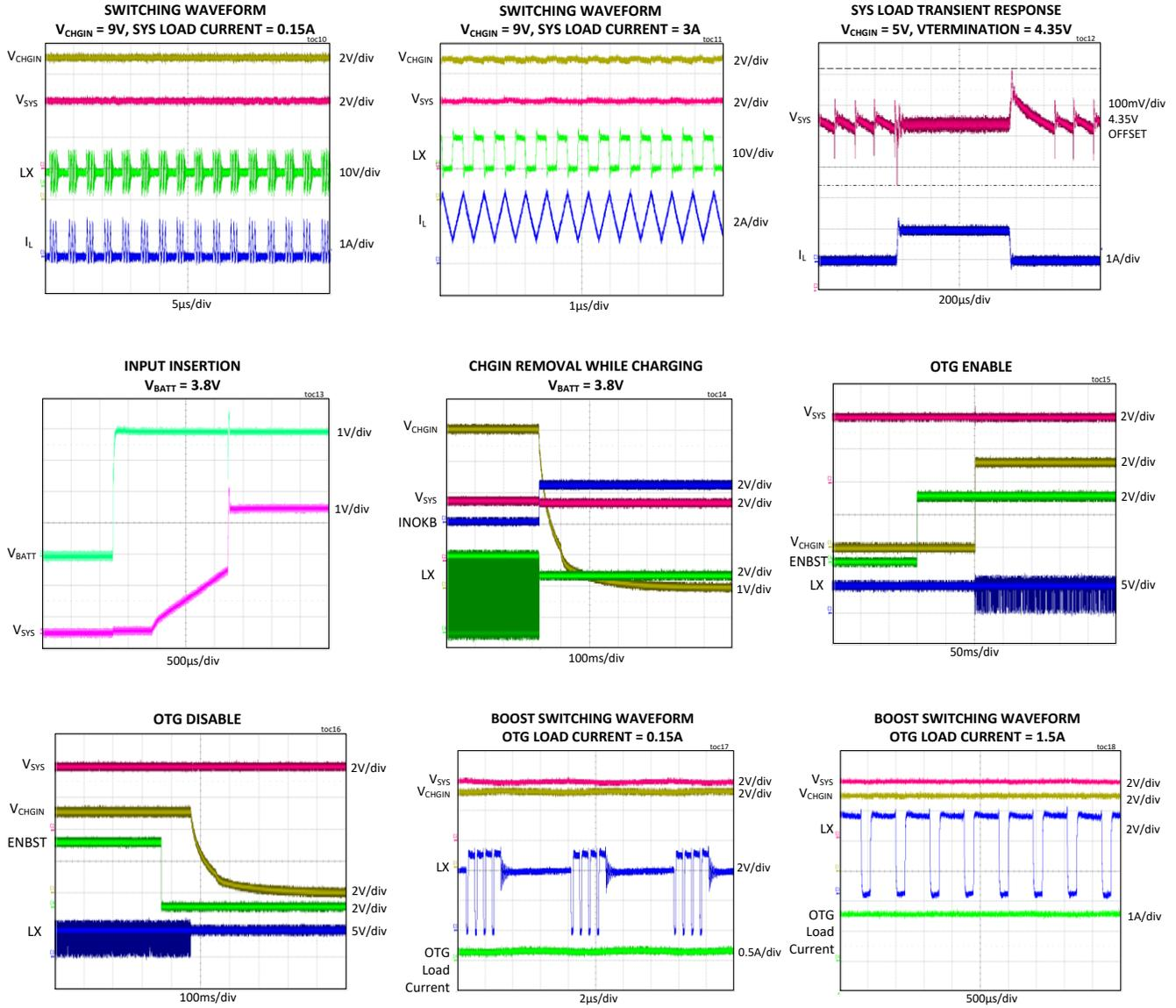
( $V_{CHGIN} = 5V$ ,  $V_{BATT} = 3.8V$ ,  $T_A = +25^\circ C$ , unless otherwise noted.)
