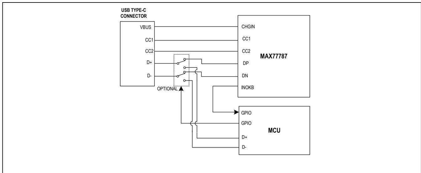
Figure 12. D+/D- Connections in a Reference System
