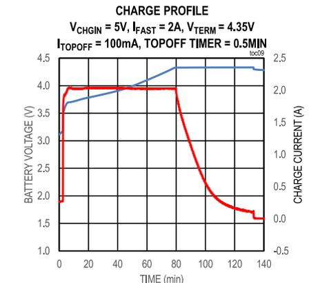
( $V_{CHGIN} = 5V$ ,  $V_{BATT} = 3.8V$ ,  $T_A = +25^\circ C$ , unless otherwise noted.)
