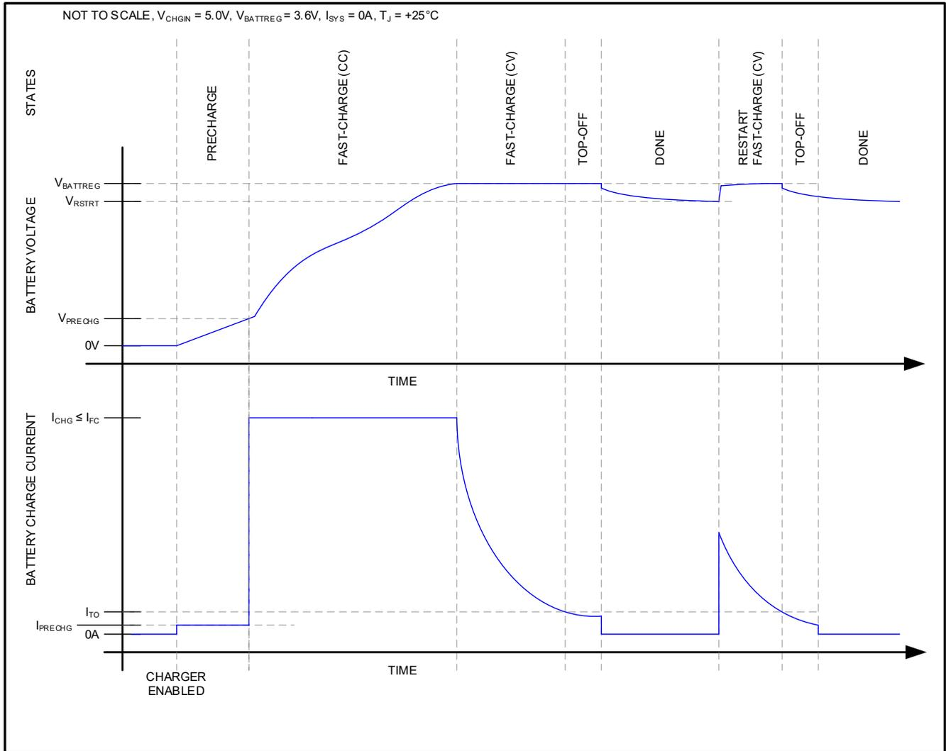
Figure 7. LiFePO<sub>4</sub> Battery Charge Profile
