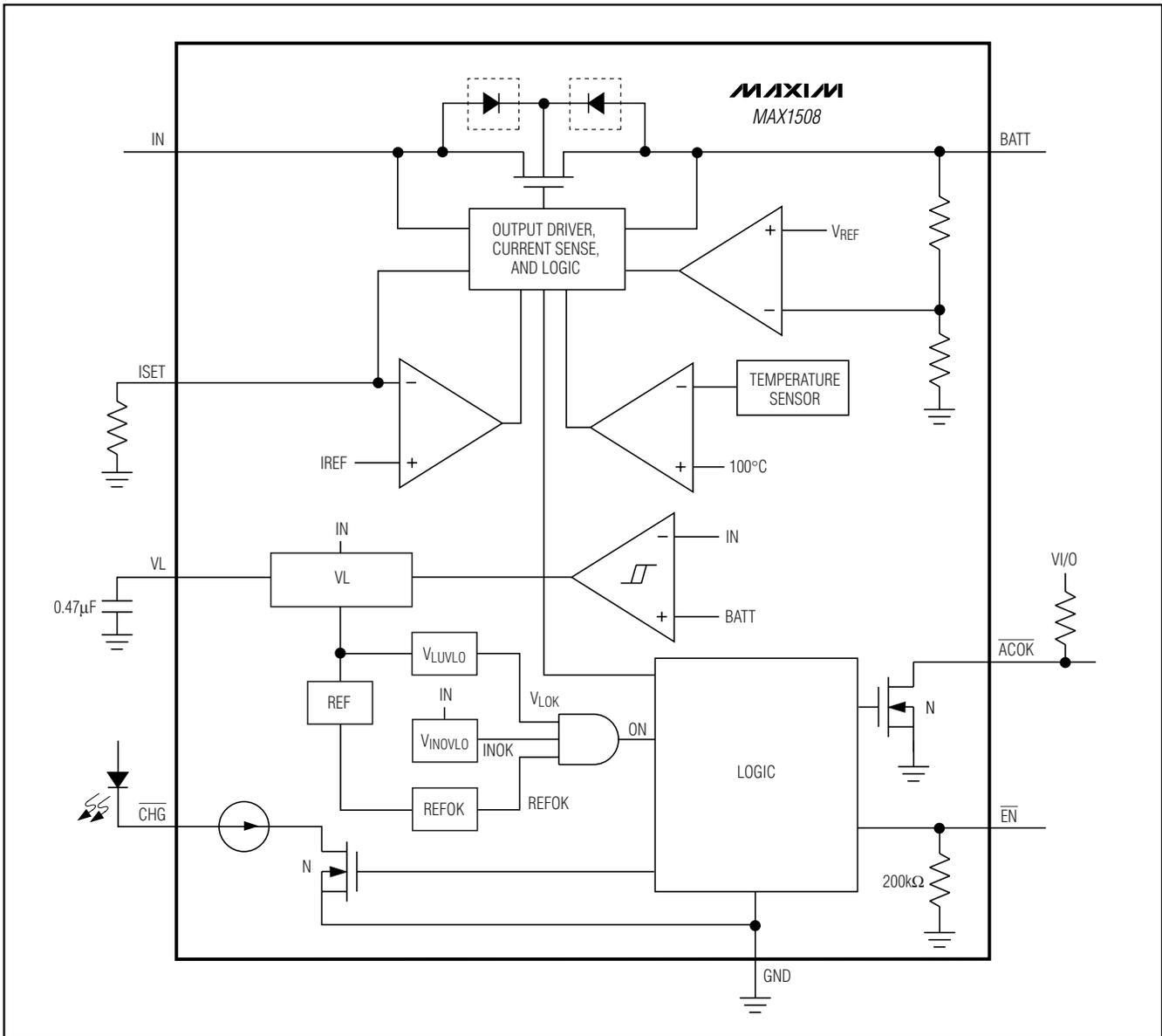
Figure 1. Functional Diagram
