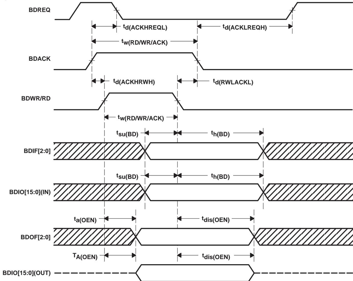
NOTE:  $t_d(\text{ACKHREQL})$  is the duration from when both BDACK and BDWR / BDRD are asserted (rising edge) until BDREQ is negated (falling edge).
