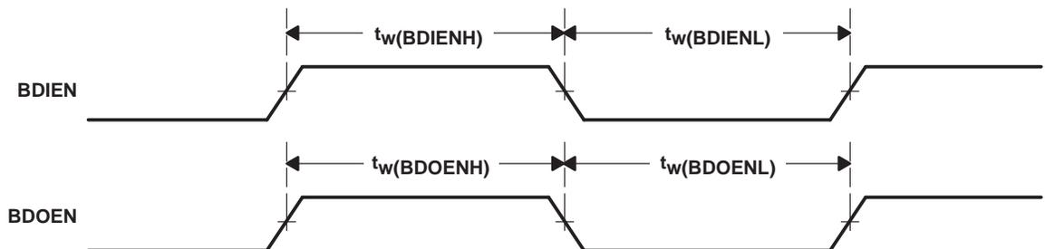
Figure 9–7. Asynchronous Mode
