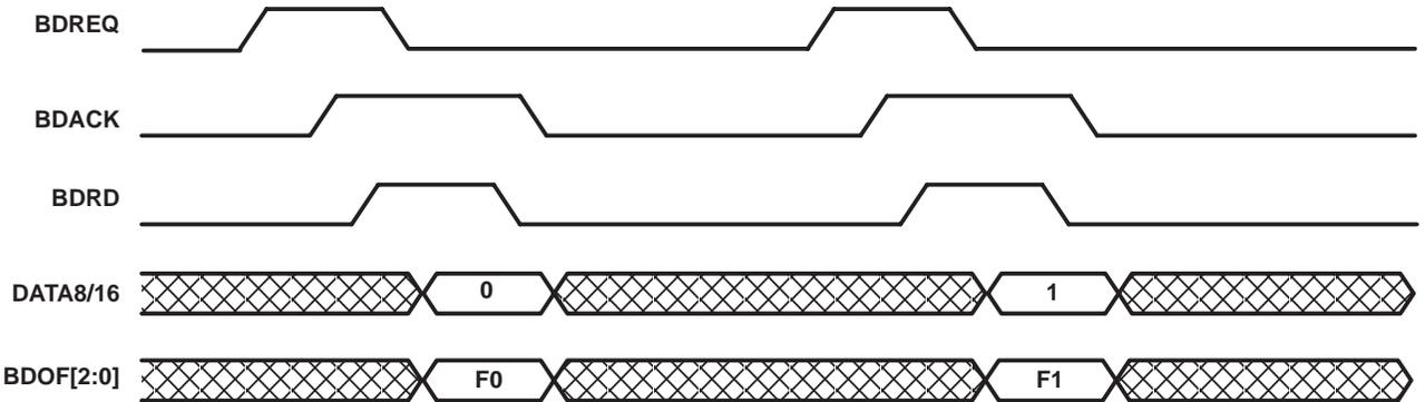
In this mode, data is output on the BDRD falling edge.
