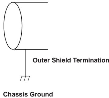
**Figure 12–2. Nonisolated Outer Shield Termination for 6-Pin Connector**
