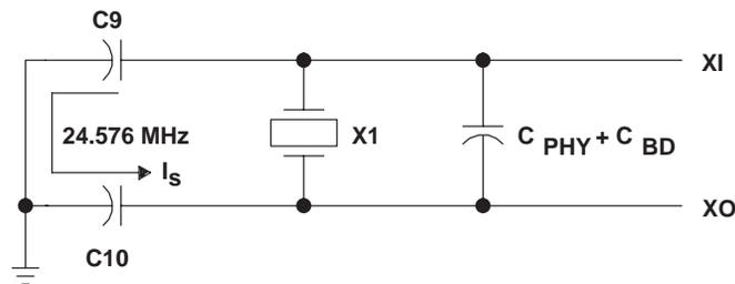
**Figure 12–4. Load Capacitance for the TSB43AA82 PHY Portion**
