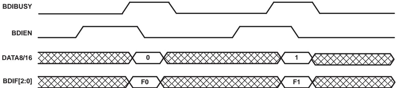
The data needs to be specified by the BDIEN falling edge. Also, BDIEN needs to be asserted after confirming BDIBUSY input is false.
