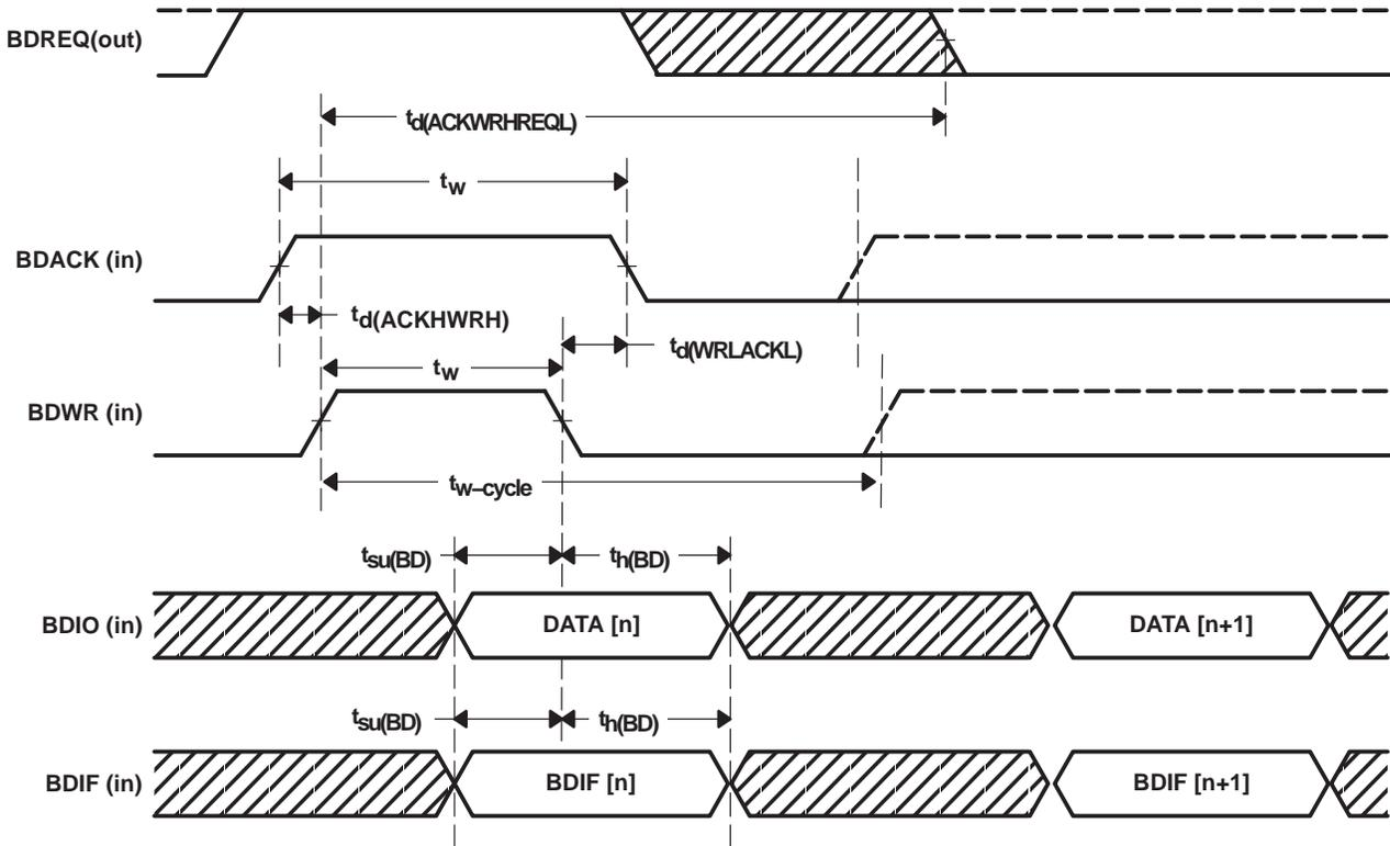
NOTE:  $t_d(\text{ACKHREQ})$  is the duration from when both BDACK and BDWR / BDRD are asserted (rising edge) until BDREQ is negated (falling edge). BDREQ remains active (asserted) while the FIFO has capacity.
