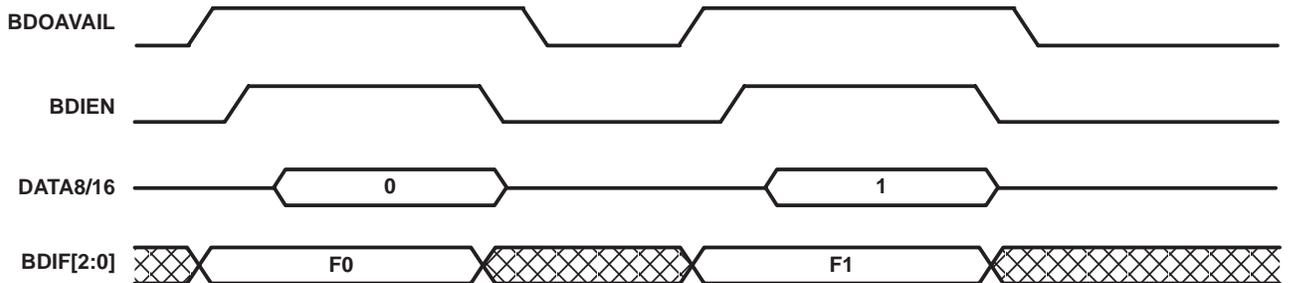
The data is output by repeating BDOEN low and high. BDOEN is asserted after confirming the BDOAVAIL input is true.
