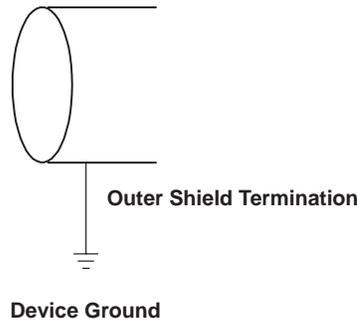
**Figure 12–3. Nonisolated Outer Shield Termination for 4-Pin Connector**
