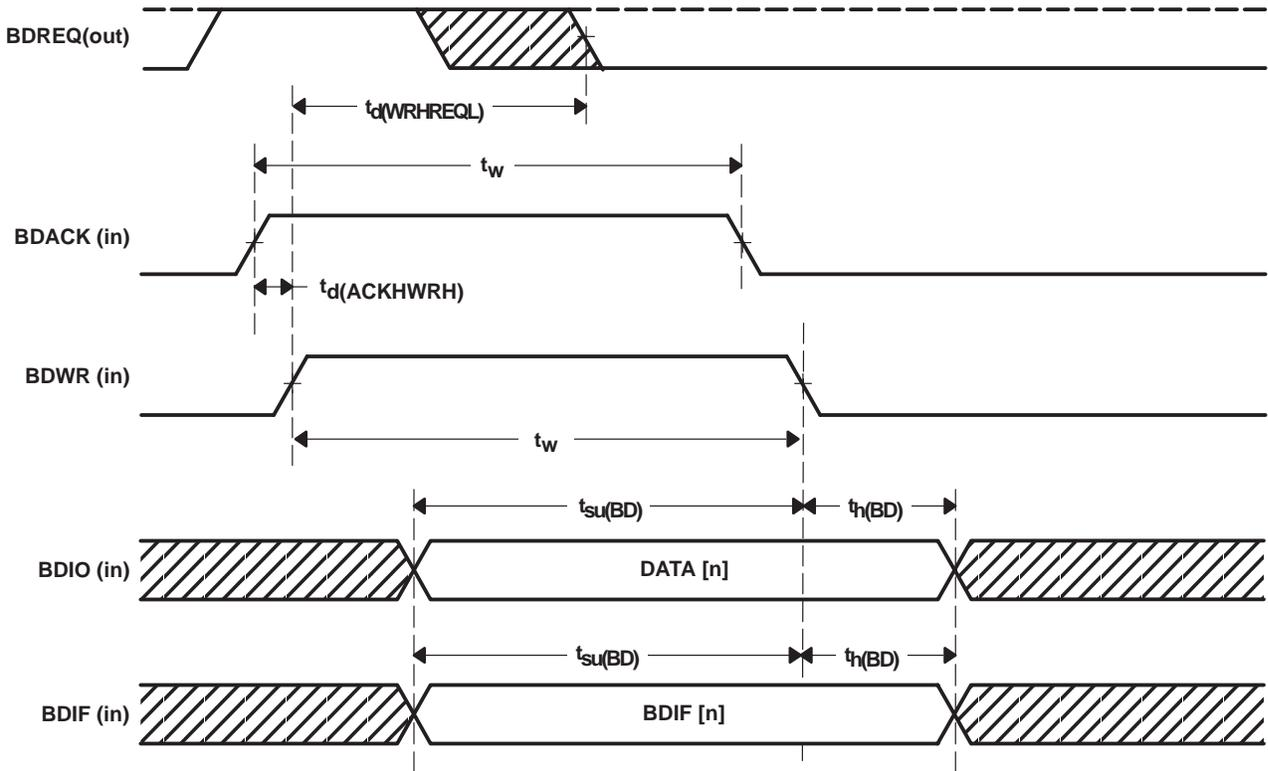
NOTE:  $t_d(ACKHREQL)$  is the duration from when both BDACK and BDWR / BDRD are asserted (rising edge) until BDREQ is negated (falling edge). BDREQ remains active (asserted) while the FIFO has capacity.
