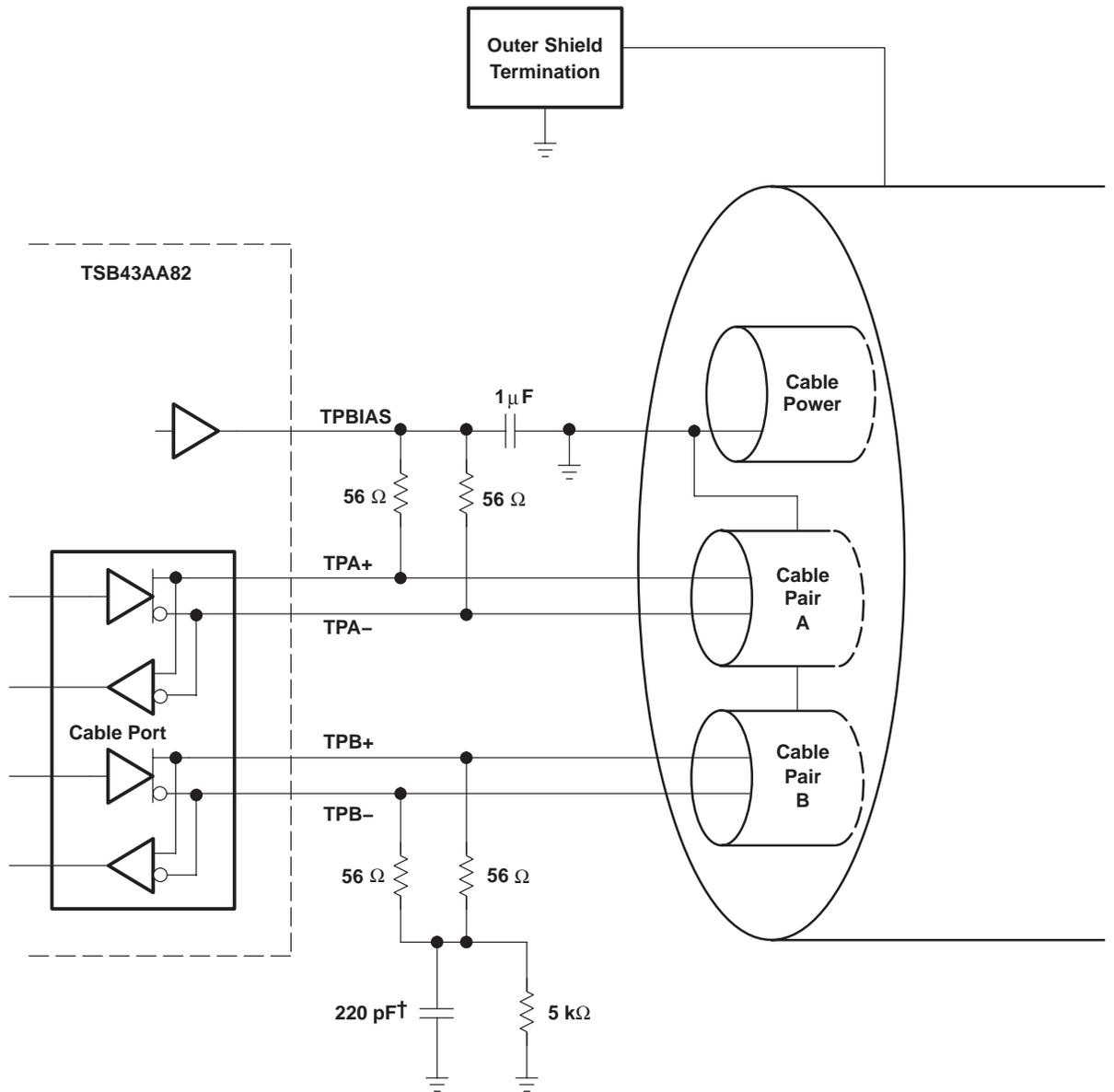
† IEEE Std 1394-1995 calls for a 250 pF capacitor, which is a nonstandard component value. A 220 pF capacitor is recommended.
