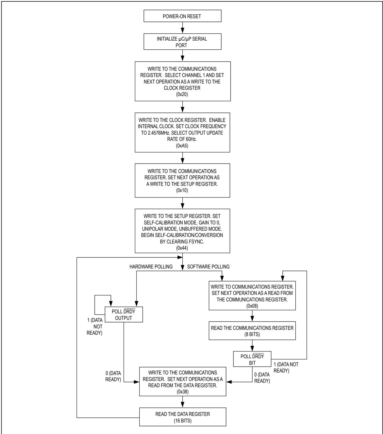
Figure 11. Sample Flow Diagram for Data Conversion
