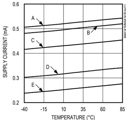
A: BUFFERED MODE  $f_{CLKIN} = 2.4576MHz$ , GAIN = 8 TO 128
