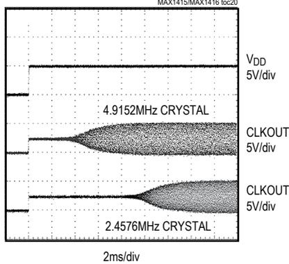
INTERNAL OSCILLATOR STARTUP TIME
