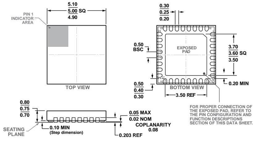
Figure 35. 32-Lead Lead Frame Chip Scale Package [LFCSP\_SS]
