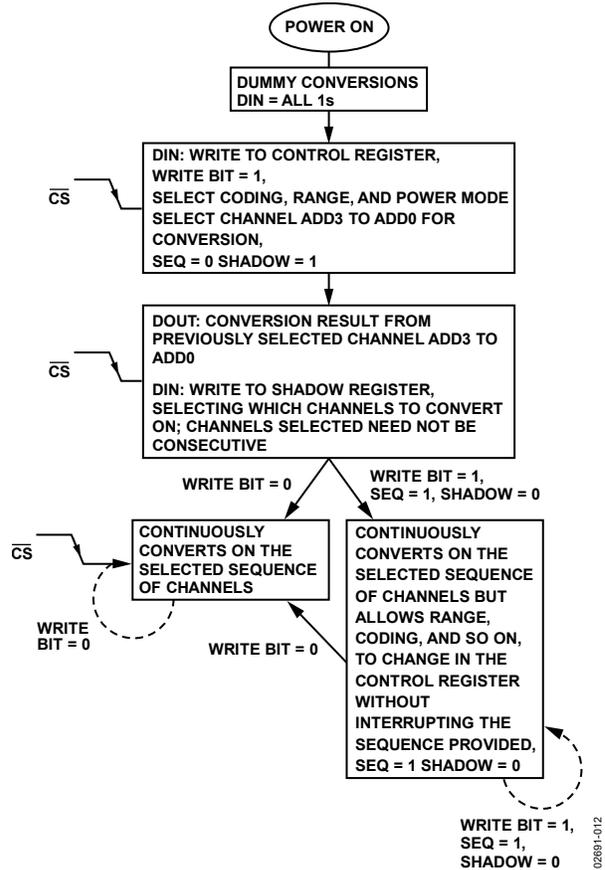
Figure 13. SEQ Bit = 0, SHADOW Bit = 1 Flowchart
