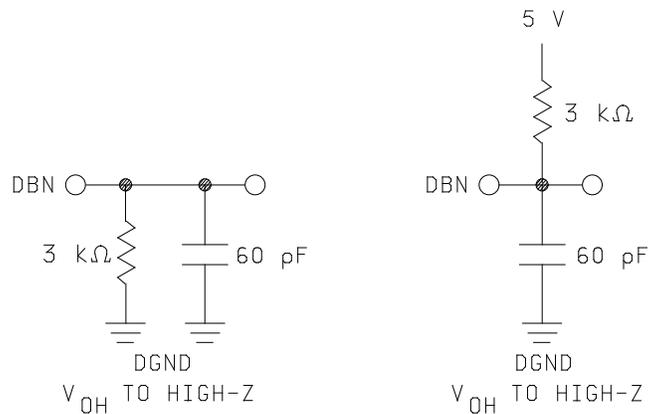
FIGURE 3. Load circuit for bus relinquish time.
