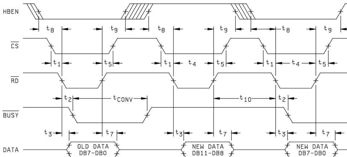
FIGURE 7. ROM mode, two byte read timing diagrams.
