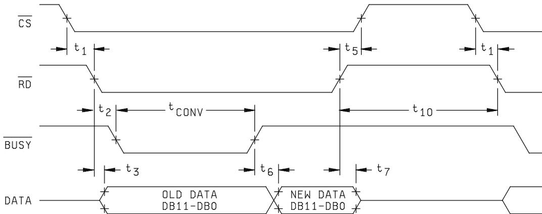
FIGURE 4. Slow memory mode, parallel read timing diagrams.
