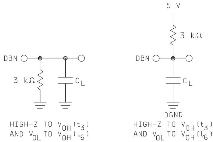
FIGURE 2. Load circuit for access time.
