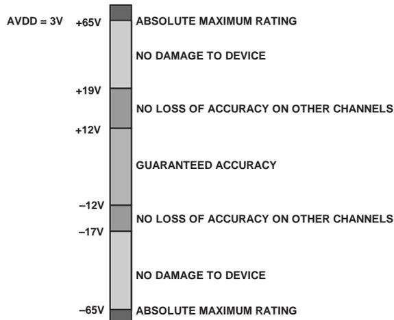
Figure 27. Absolute Input Pin Voltages, AVDD = 3 V
