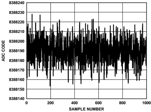
Figure 6. Noise (Output Data Rate = 2.5 kSPS)
