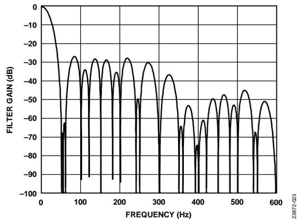
Figure 37. 25 SPS ODR, 40 ms Settling Time
