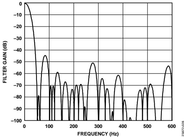
Figure 42. 16.667 SPS ODR, 60 ms Settling Time
