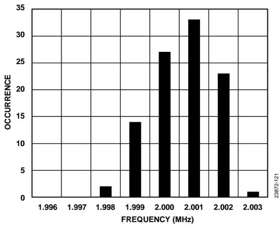
Figure 13. Internal Oscillator Frequency and Accuracy Distribution Histogram
