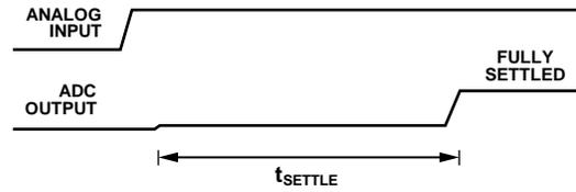
Figure 35. Step Input with Single Cycle Settling
