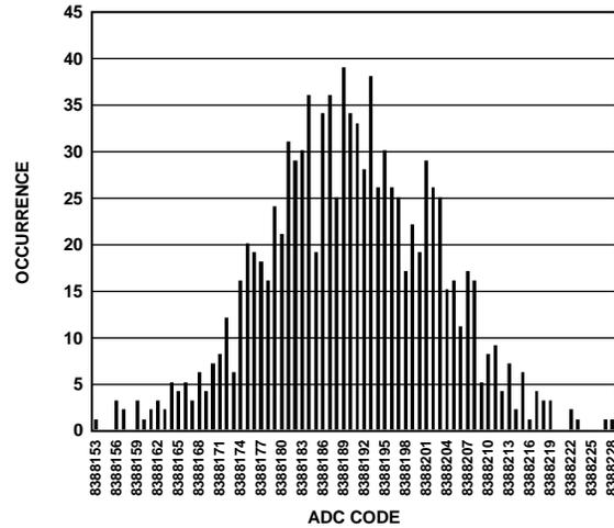
Figure 9. Histogram (Output Data Rate = 2.5 kSPS)
