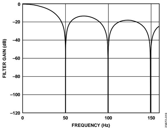
Figure 32. Sinc5 + Sinc1 Filter Response at 50 SPS ODR
