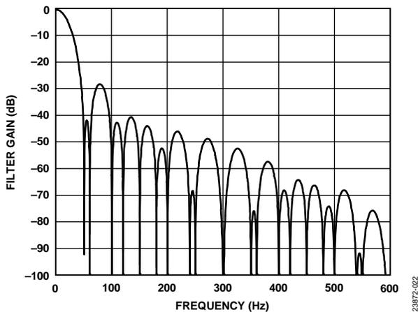
Figure 36. 27.27 SPS ODR, 36.67 ms Settling Time
