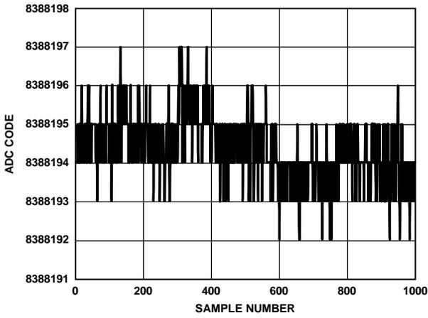
Figure 5. Noise (Output Data Rate = 1.25 SPS)
