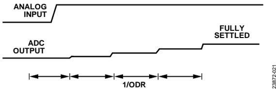
Figure 34. Step Input Without Single Cycle Settling
