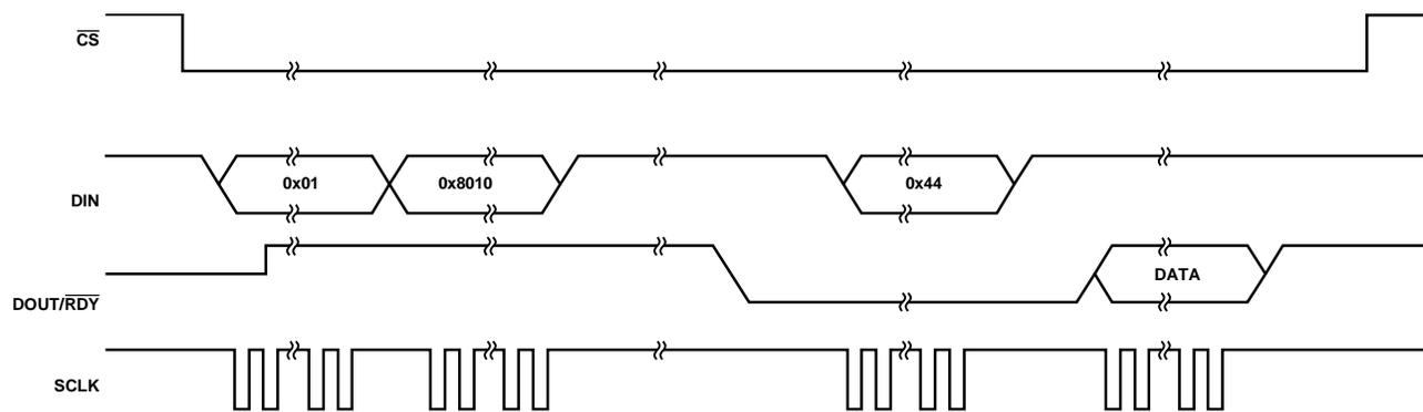
Figure 46. SPI Communication in Single Conversion Mode
