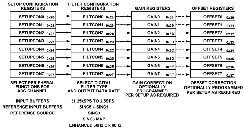
Figure 25. ADC Setup Register Grouping
