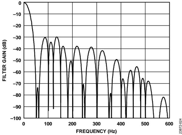
Figure 38. 20 SPS ODR, 50 ms Settling Time
