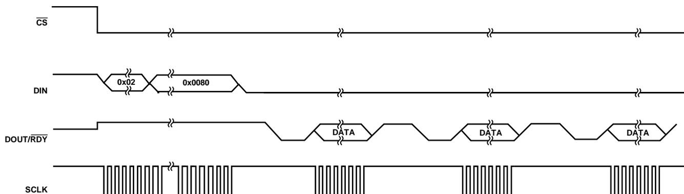
Figure 45. SPI Communication in Continuous Read Mode
