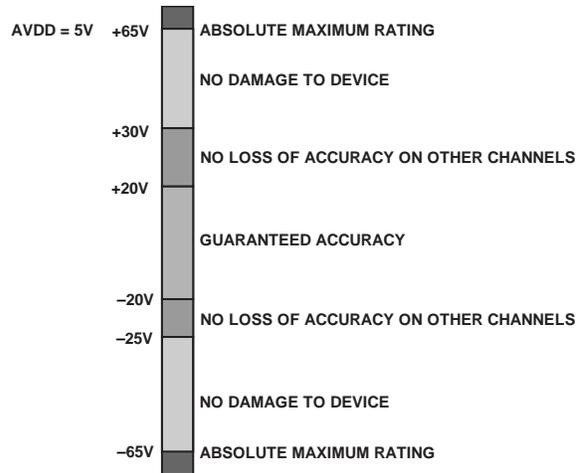
Figure 28. Absolute Input Pin Voltages, AVDD = 5 V
