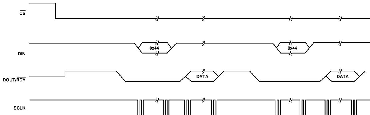
Figure 44. SPI Communication in Continuous Conversion Mode
