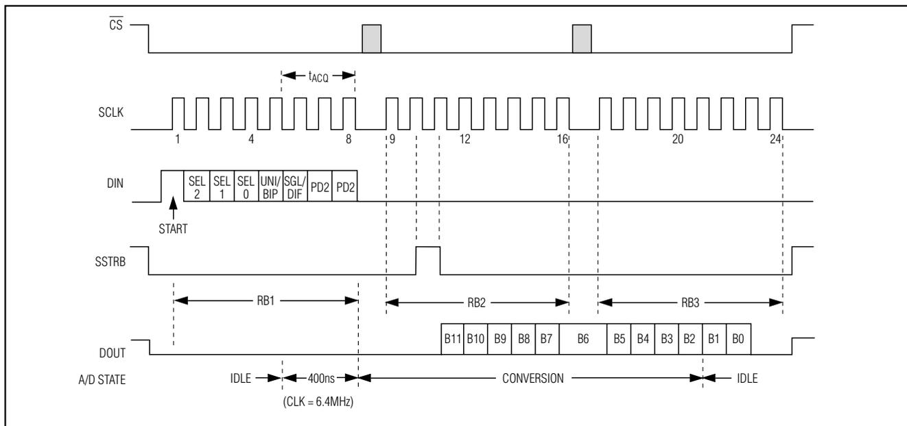
Figure 5. Single-Conversion Timing
