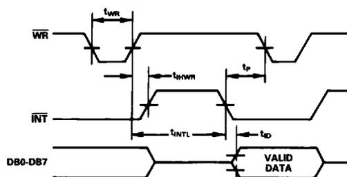
Figure 6. WR-RD Mode Stand-Alone Operation, CS = RD = 0
