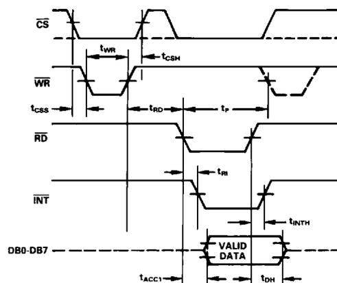
Figure 5b. WR-RD Mode (t<sub>RD</sub> < t<sub>INTL</sub>)
