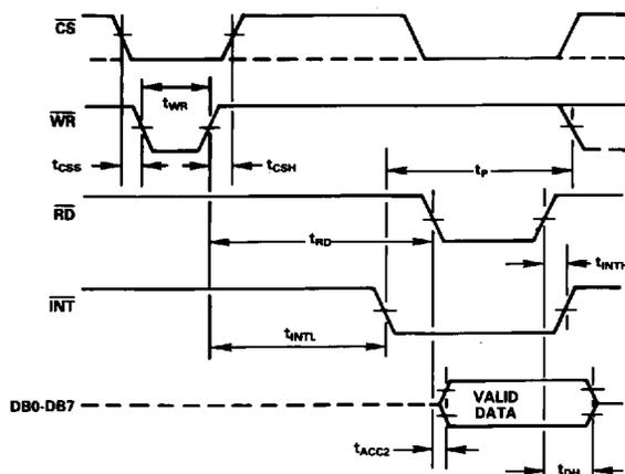
Figure 5a. WR-RD Mode (t<sub>RD</sub> > t<sub>INTL</sub>)
