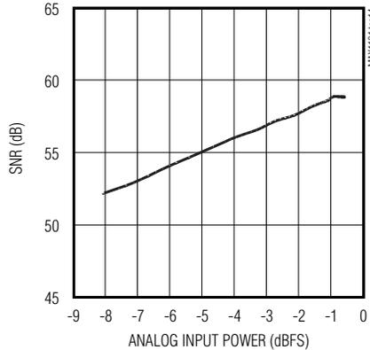
**SIGNAL-TO-NOISE AND DISTORTION vs. ANALOG INPUT POWER ( $f_{IN} = 20\text{MHz}$ )**
