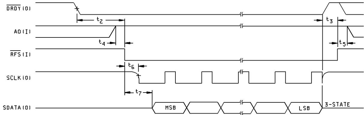
Self-clocking mode, output data read operation
