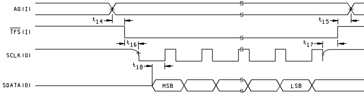
Self-clocking mode, control/calibration register write operation
