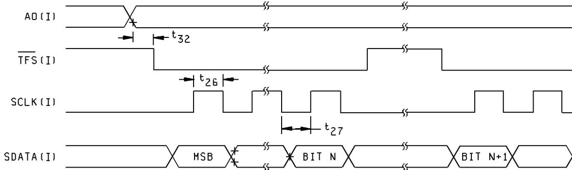
External-clocking mode, control/calibration register write operation (TFS returns high during write operation)
