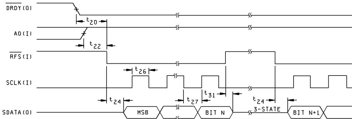
External-clocking mode, output data read operation (RFS returns high during read operation)
