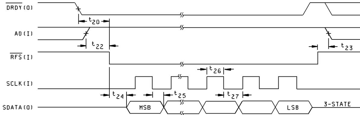
External-clocking mode, output data read operation
