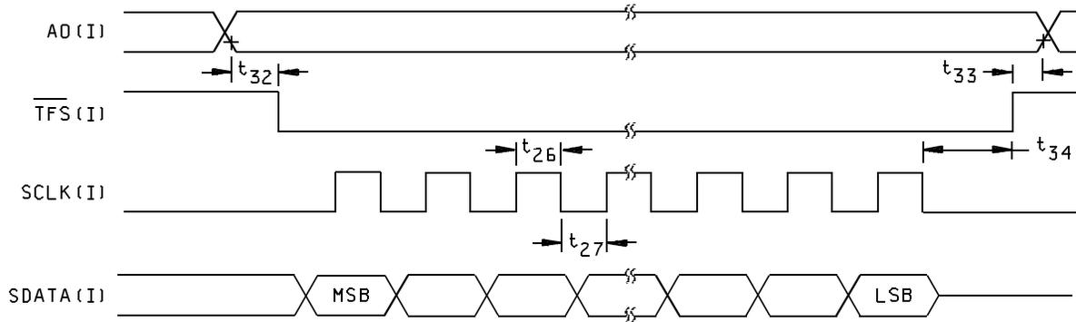
External-clocking mode, control/calibration register write operation
