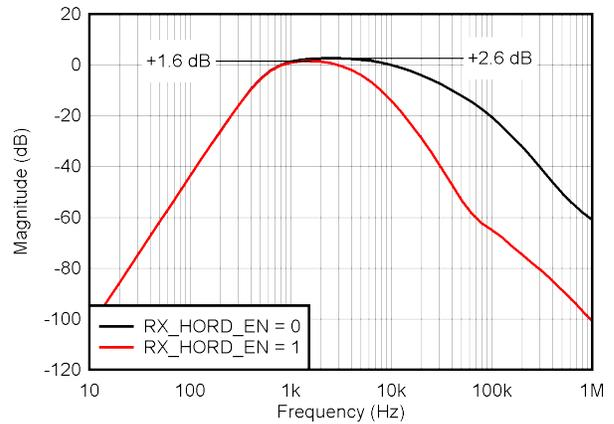
2.2 nF HART\_RX Input Capacitor      680 pF RX\_INF Capacitor to Ground
