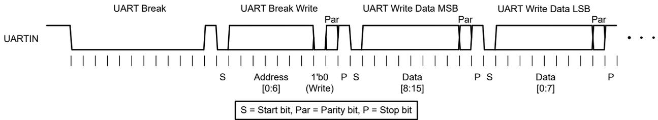
**Figure 6-31. UARTIN Break Write Data Format**
