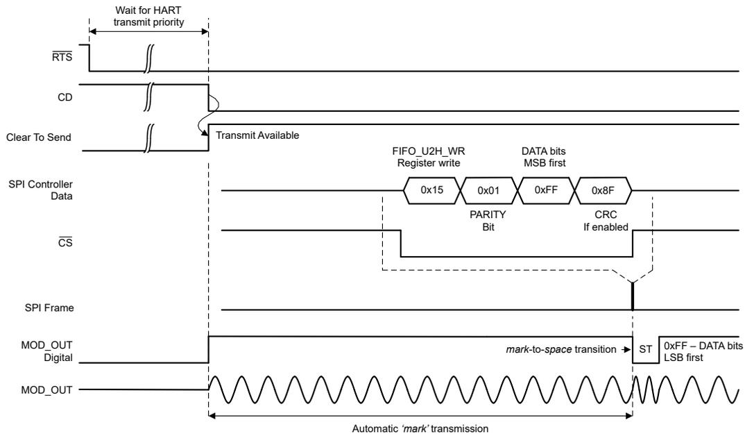
**Figure 6-21. HART Transmit Start Timing Diagram (SPI Mode)**
