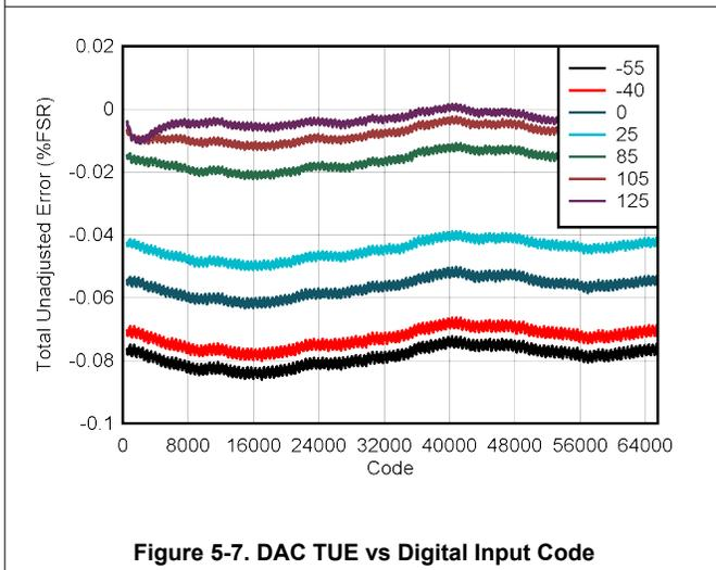
**Figure 5-7. DAC TUE vs Digital Input Code**
