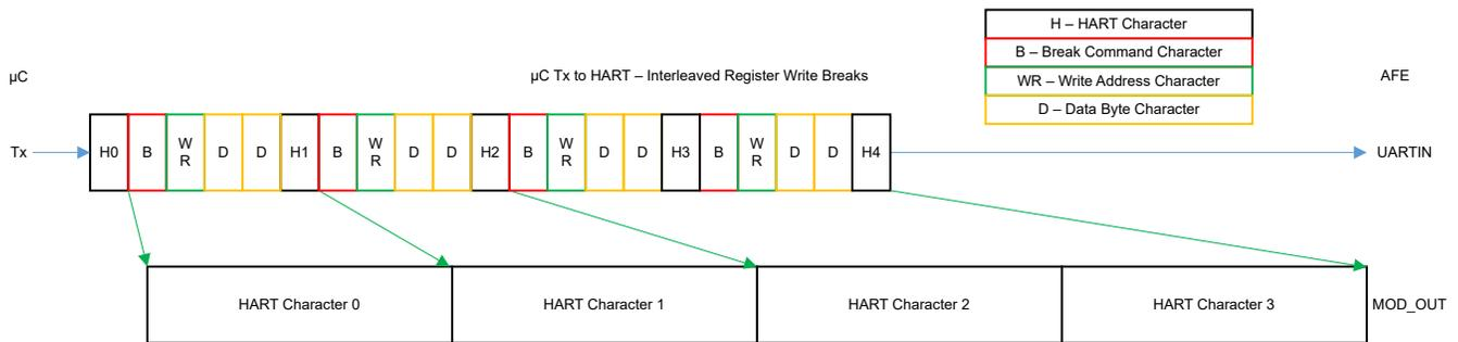
**Figure 6-34. Interleaved HART Transmit With UBM Register Writes**
