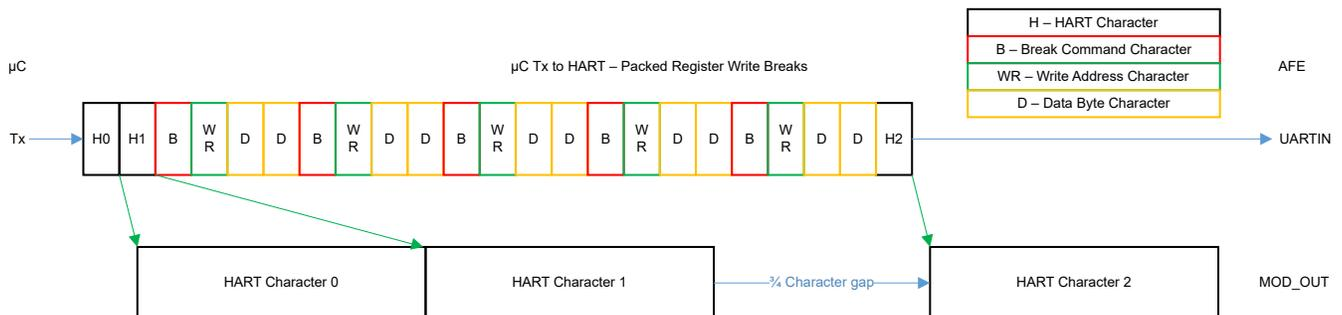
**Figure 6-35. Packed HART Transmit With UBM Register Writes**
