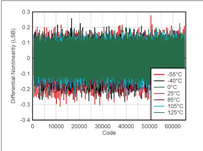
**Figure 5-3. DAC DNL vs Digital Input Code**
