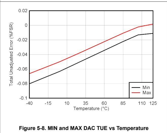
**Figure 5-8. MIN and MAX DAC TUE vs Temperature**
