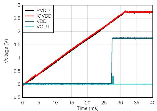
Figure 5-26. DAC Supply Power On, PVDD = 2.7 V
