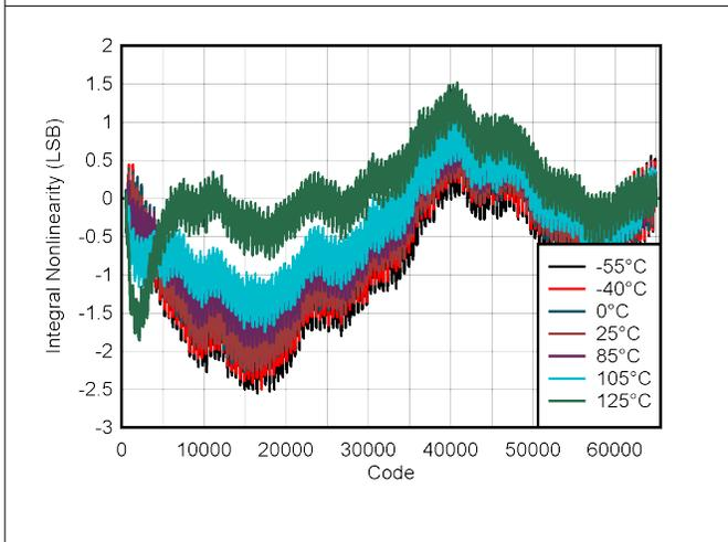
**Figure 5-5. DAC INL vs Digital Input Code**
