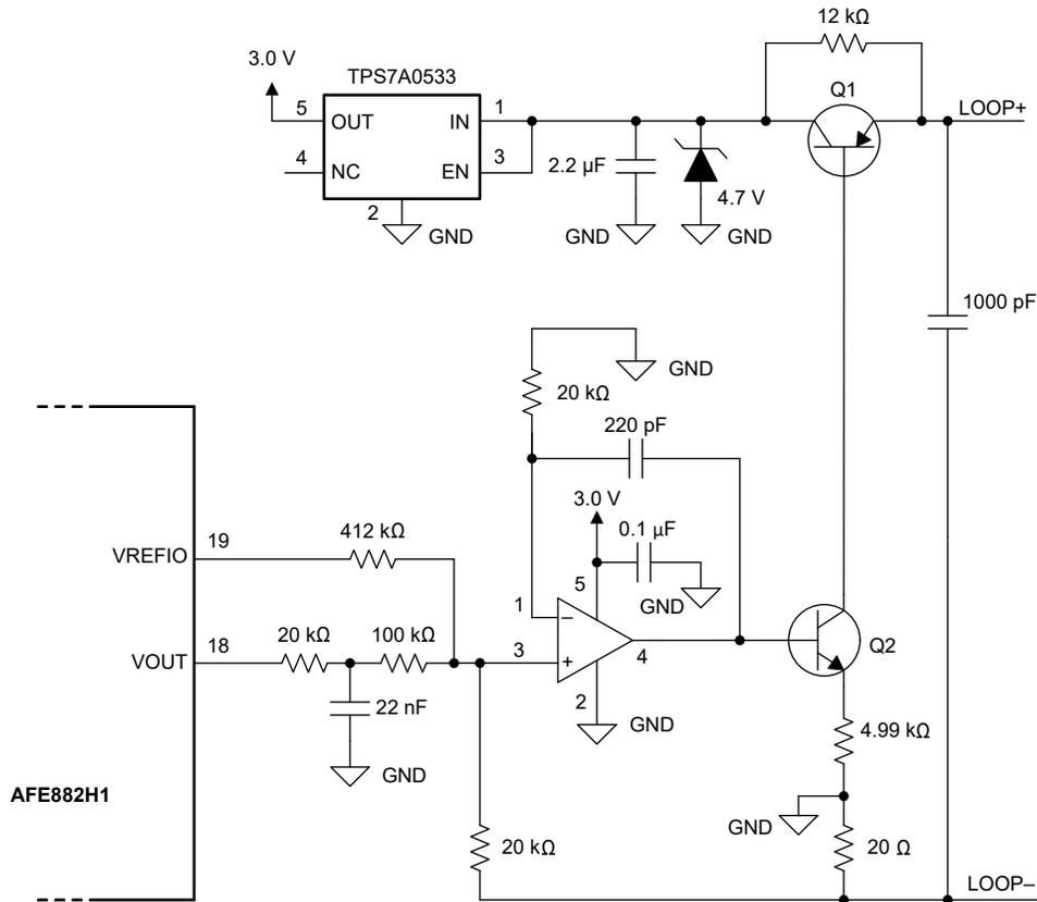
**Figure 8-4. Current Loop Control for the AFE882H1 Transmitter**
