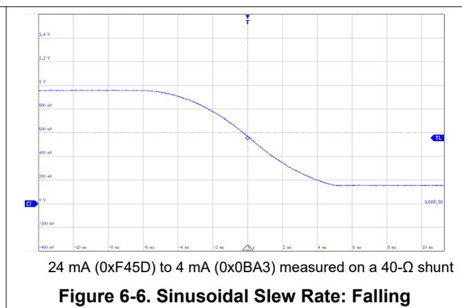
If the slew-rate feature is disabled while the DAC is executing the slew-rate command, the slew-rate operation is aborted, and the DAC output goes to the target code.
