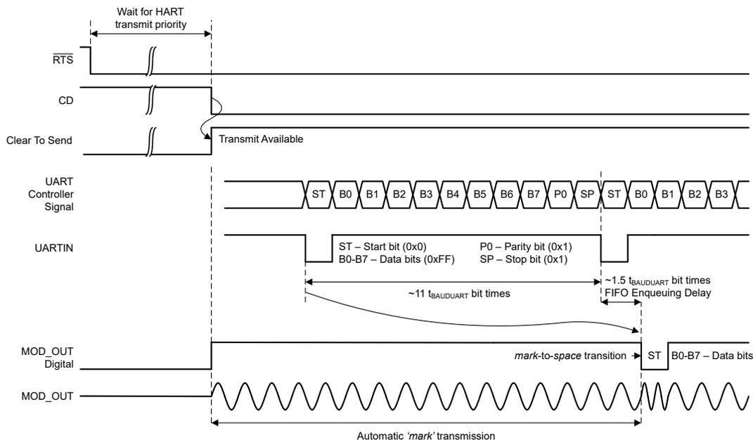
**Figure 6-20. HART Transmit Start Timing Diagram (UART Mode)**
