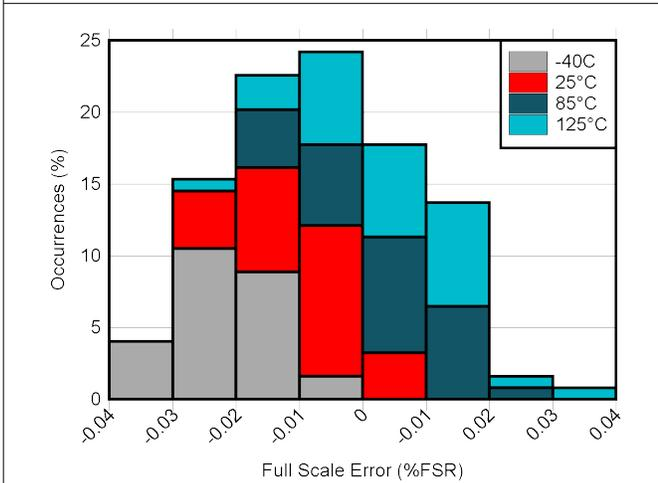
**Figure 5-17. DAC Full Scale Error vs Temperature**
