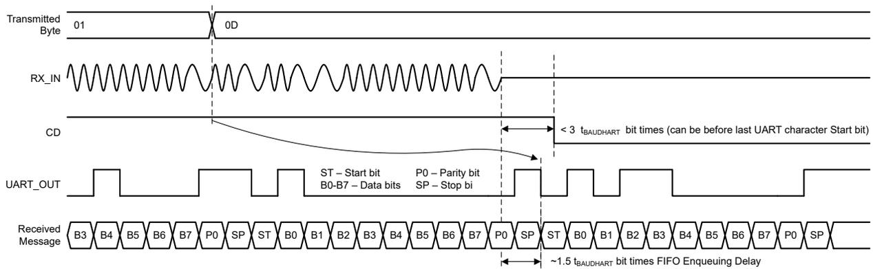
**Figure 6-24. HART Receive End Timing Diagram (UART Mode)**
