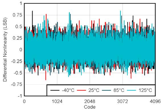
Figure 5-28. ADC DNL vs Digital Input Code
