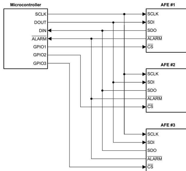
**Figure 8-1. Multichannel Configuration**
