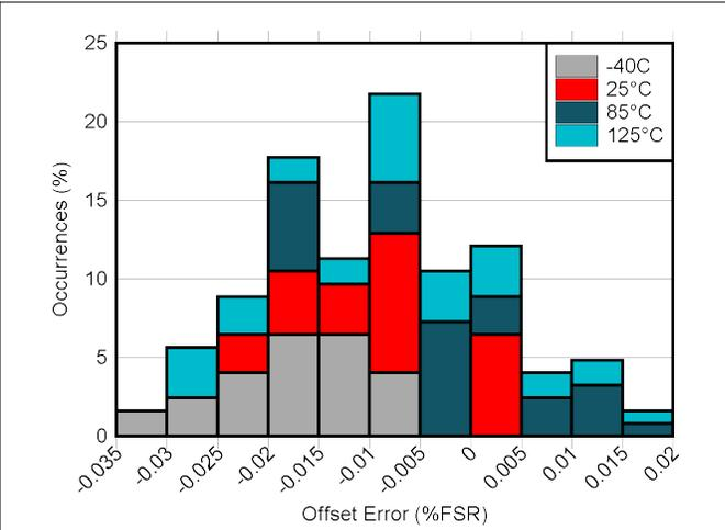
**Figure 5-16. DAC Offset Error vs Temperature**
