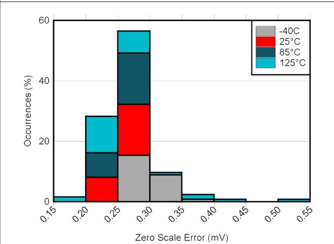
**Figure 5-18. DAC Zero Scale Error vs Temperature**
