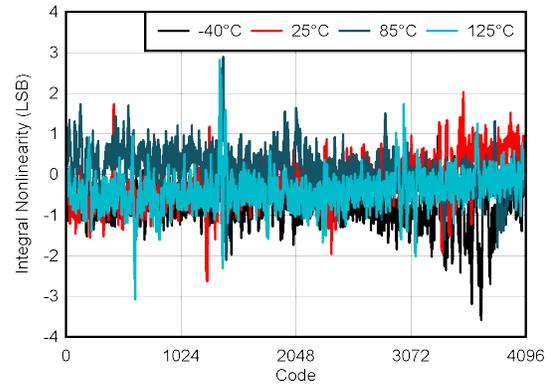
Figure 5-29. ADC INL vs Digital Input Code
