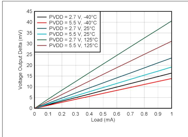
Figure 5-9. Zero-code Impedance
