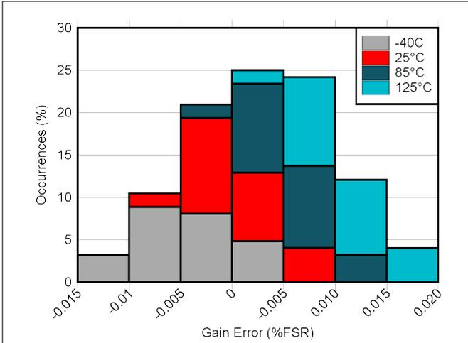
**Figure 5-15. DAC Gain Error vs Temperature**
