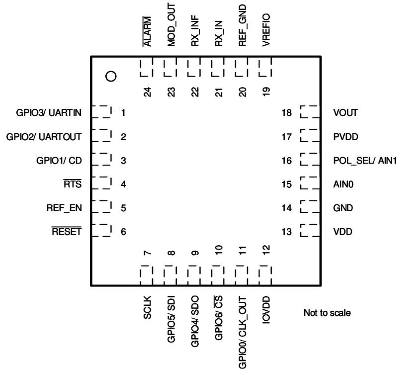
Figure 4-1. RRU Package, 24-pin UQFN (Top View)
