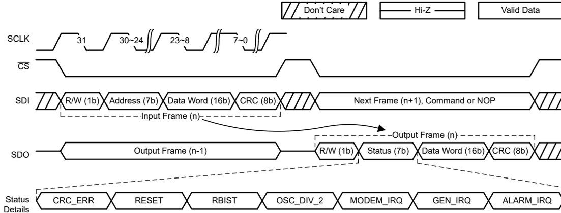
Figure 6-29. SPI Frame Details (Default, CRC Enabled)
