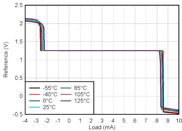
Figure 5-42. Reference Source and Sink Current Capability
