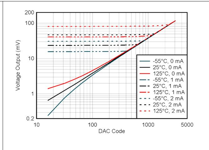
Figure 5-10. DAC Footroom Over Temperature and Load
