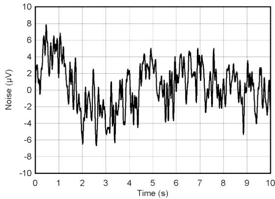
Figure 5-40. Reference Output Noise, 0.1 Hz to 10 Hz
