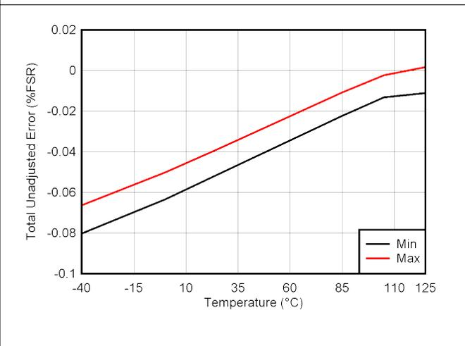
Figure 6-8. MIN and MAX DAC TUE vs Temperature
