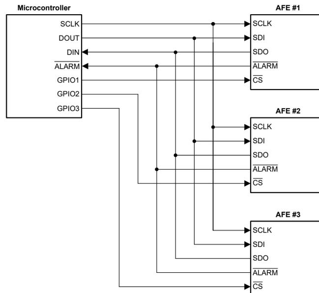
**Figure 8-1. Multichannel Configuration**
