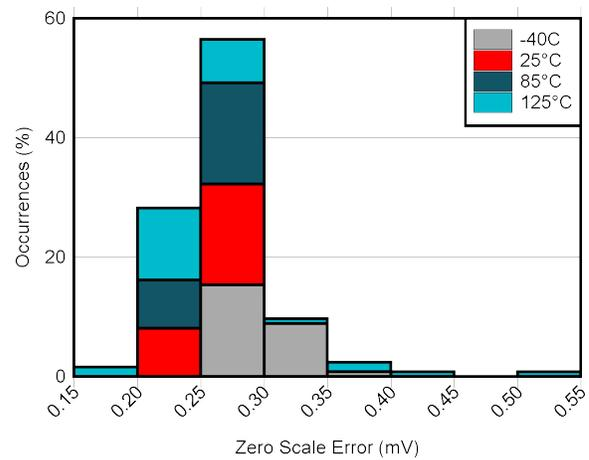
Figure 6-18. DAC Zero Scale Error vs Temperature
