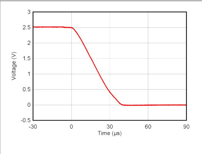
**Figure 6-22. DAC Falling Settling Time**
