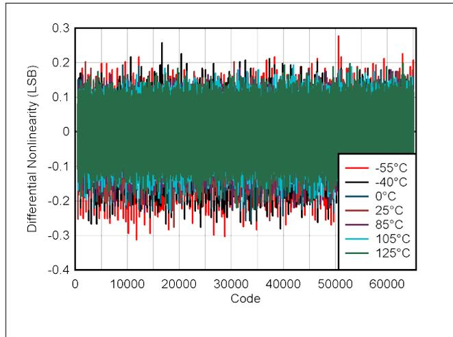
Figure 6-3. DAC DNL vs Digital Input Code
