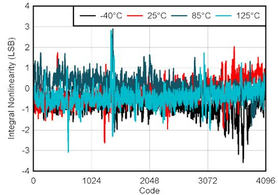
**Figure 6-29. ADC INL vs Digital Input Code**
