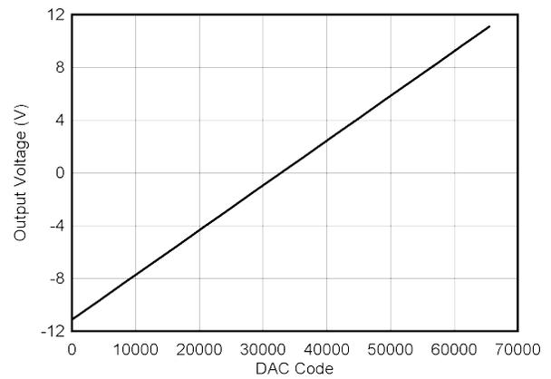
**Figure 8-7. DAC Code to XTR Output Voltage**
