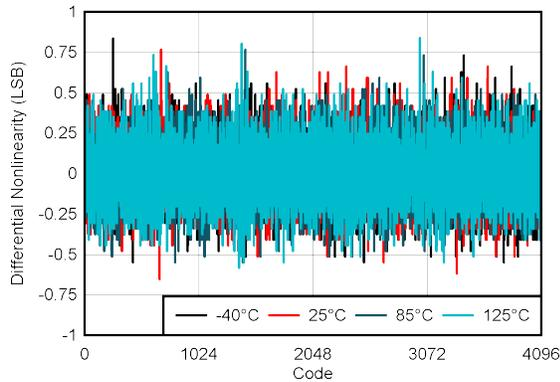
**Figure 6-28. ADC DNL vs Digital Input Code**
