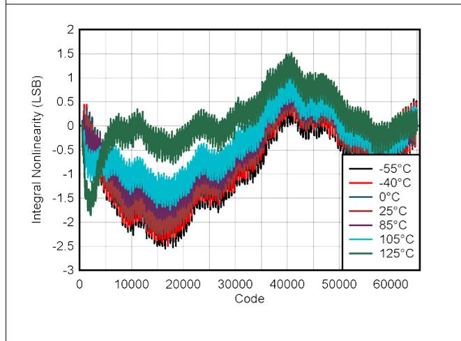
Figure 6-5. DAC INL vs Digital Input Code
