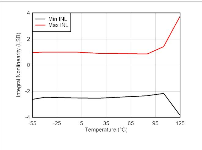
Figure 6-6. MIN and MAX DAC INL Range vs Temperature
