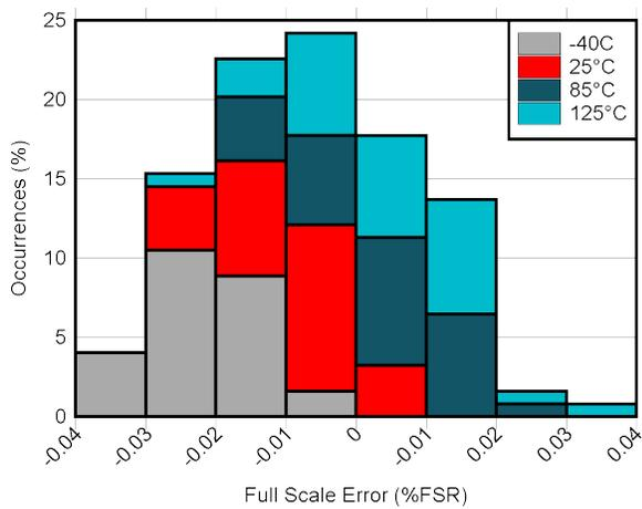
Figure 6-17. DAC Full Scale Error vs Temperature
