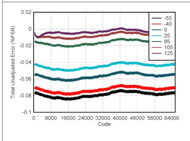
Figure 6-7. DAC TUE vs Digital Input Code
