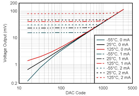
**Figure 6-10. DAC Footroom Over Temperature and Load**
