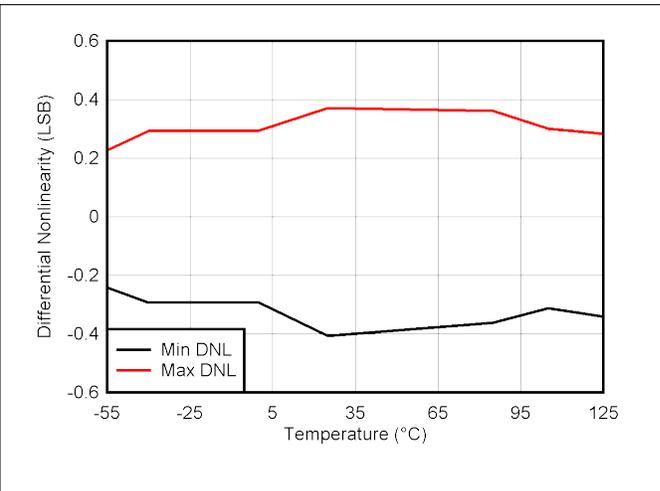
Figure 6-4. MIN and MAX DAC DNL Range vs Temperature
