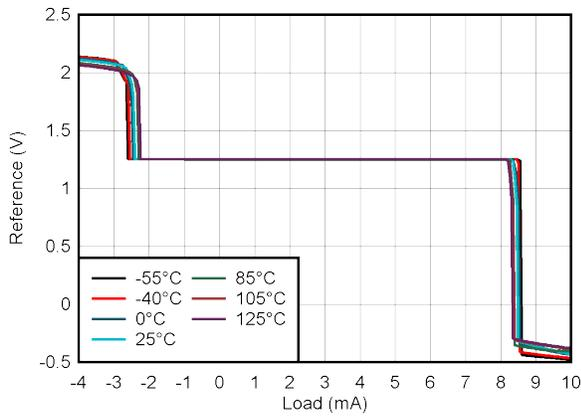
**Figure 6-42. Reference Source and Sink Current Capability**
