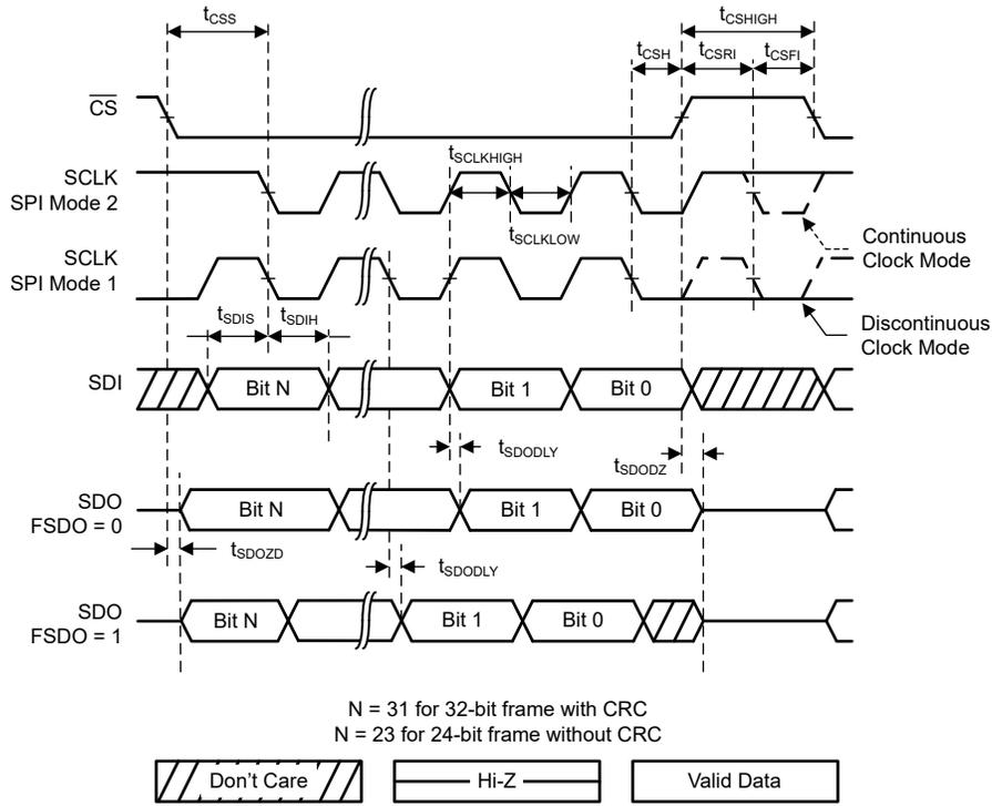
**Figure 6-1. SPI Timing**
