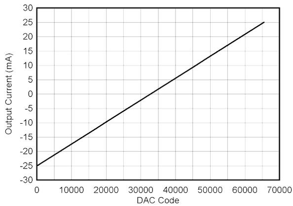
**Figure 8-6. DAC Code to XTR Output Current**
