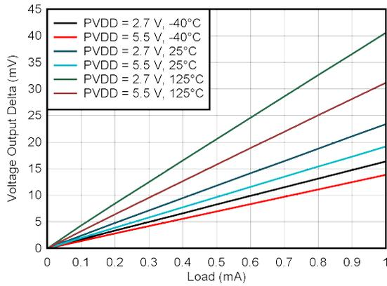
**Figure 6-9. Zero-code Impedance**
