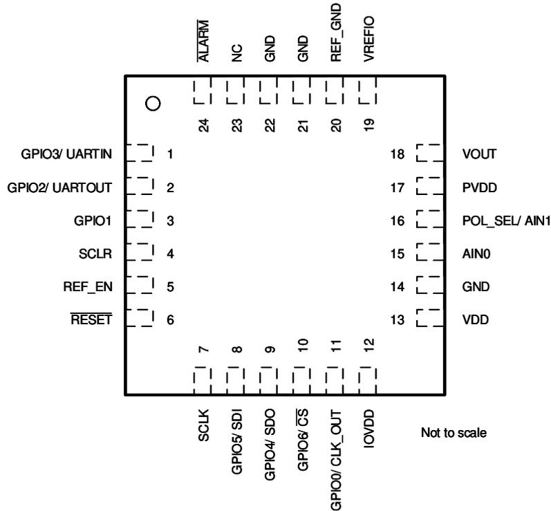
Figure 5-1. RRU Package, 24-pin UQFN (Top View)
