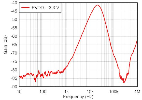
**Figure 6-41. Reference AC PSRR vs frequency**
