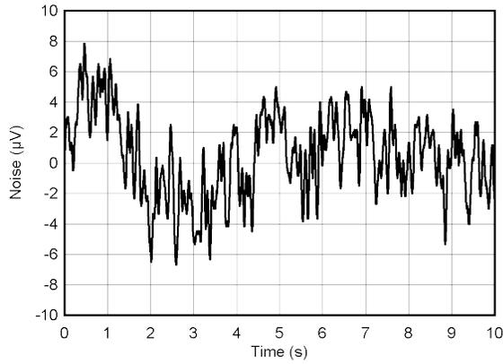
**Figure 6-40. Reference Output Noise, 0.1 Hz to 10 Hz**
