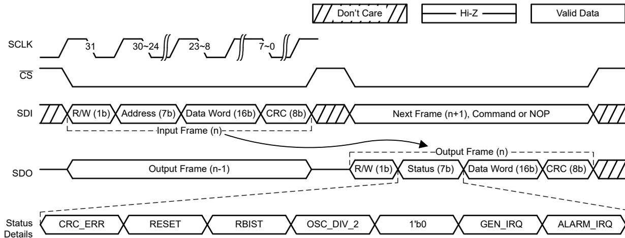
**Figure 7-19. SPI Frame Details (Default, CRC Enabled)**
