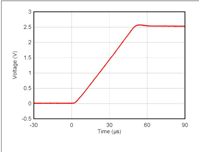
**Figure 6-21. DAC Rising Settling Time**
