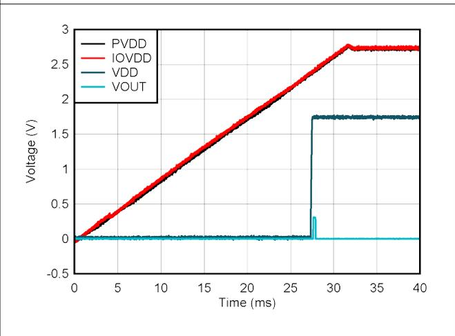
**Figure 6-26. DAC Supply Power On, PVDD = 2.7 V**
