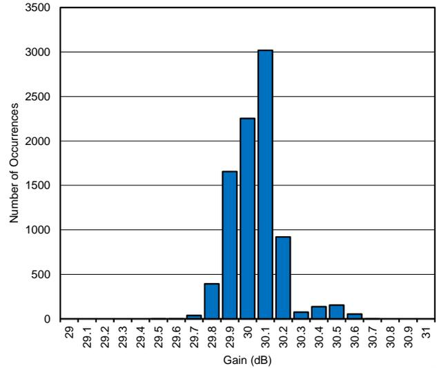
Figure 2. GAIN-MATCHING HISTOGRAM (Gain = 30 dB)
