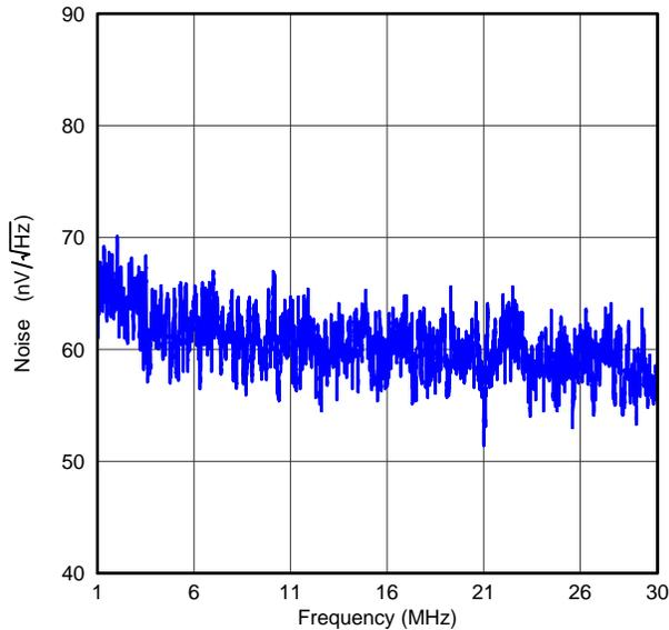
Figure 9. OUTPUT-REFERRED NOISE vs FREQUENCY (Gain = 30 dB) G010
