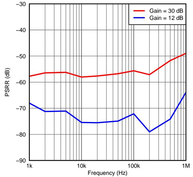
**Figure 17. POWER-SUPPLY REJECTION RATIO (100-mV<sub>PP</sub> Supply Noise with Different Frequencies)**
