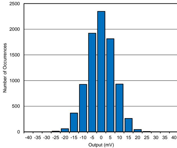
Figure 3. OUTPUT OFFSET HISTOGRAM (Gain = 30 dB)
