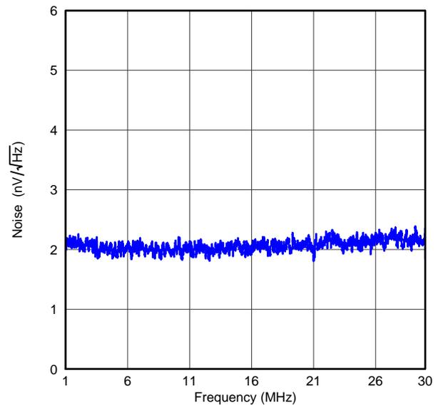
Figure 8. INPUT-REFERRED NOISE vs FREQUENCY (Gain = 30 dB)
