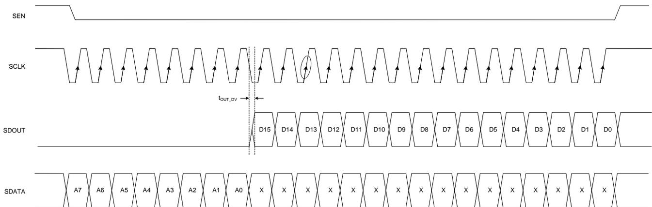
**Figure 19. Serial Interface Register Read Timing Diagram**
