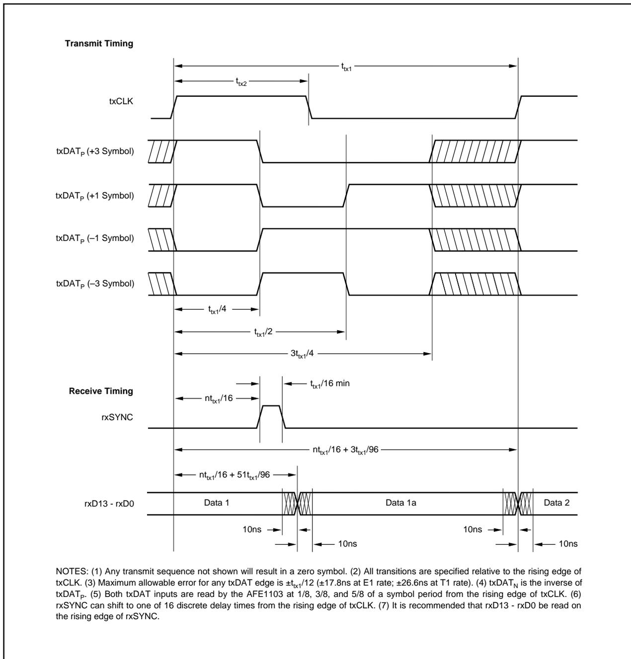
FIGURE 3. Timing Diagram.
