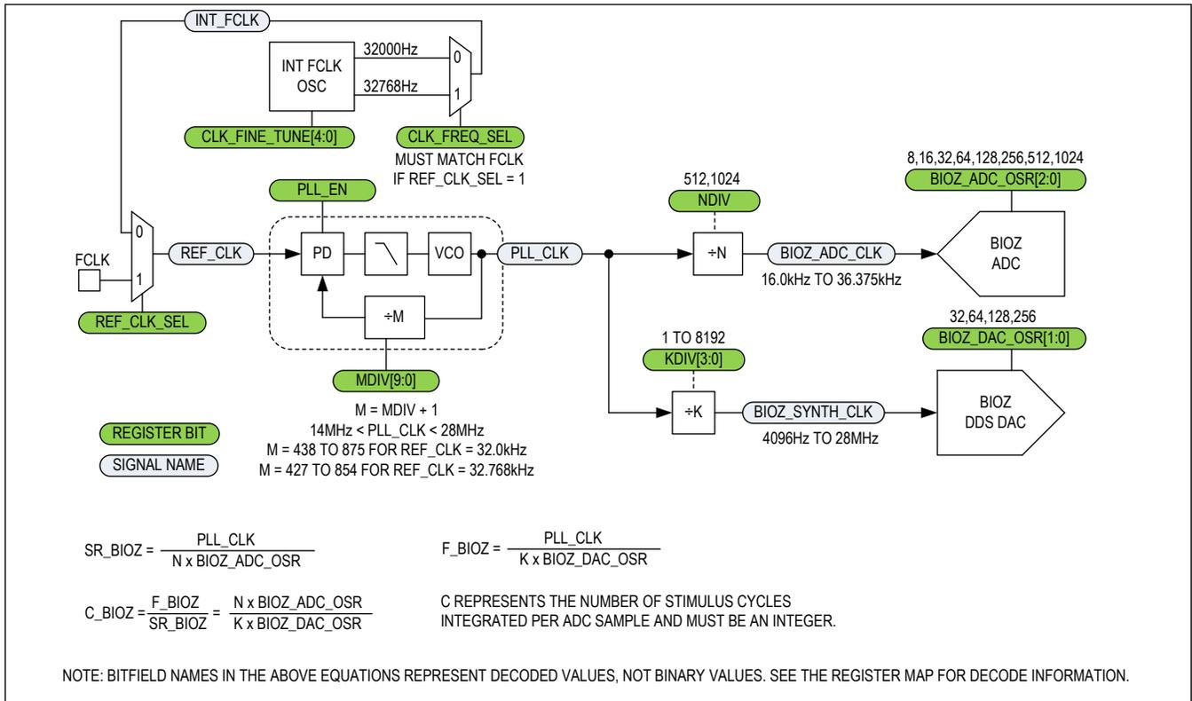
Figure 1. Timing Subsystem
