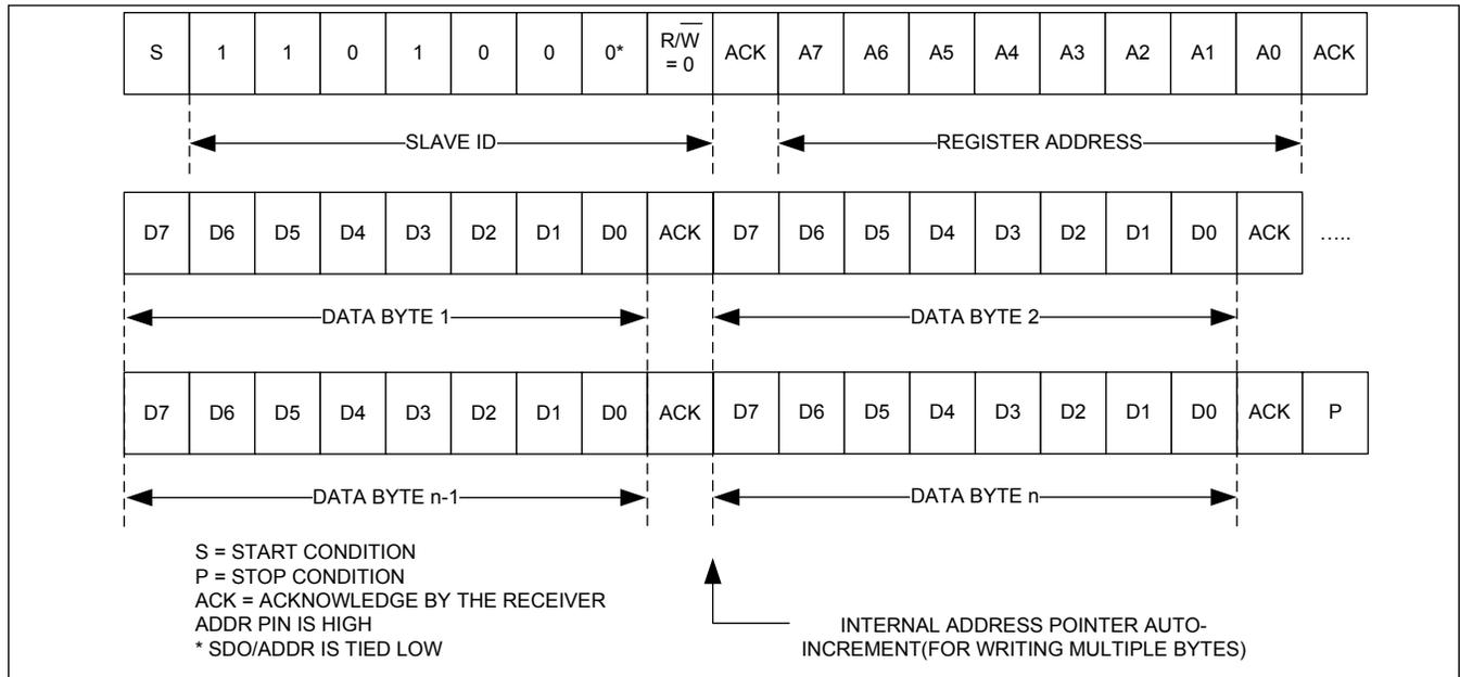
Figure 26. I<sup>2</sup>C Multibyte Write Transaction
