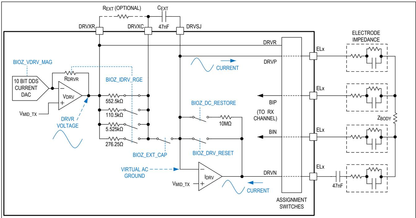
Figure 7. Bioimpedance Stimulus Generator — Sine-Wave Current Mode
