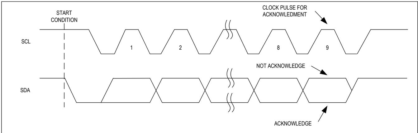
Figure 24. I<sup>2</sup>C Acknowledge Bit
