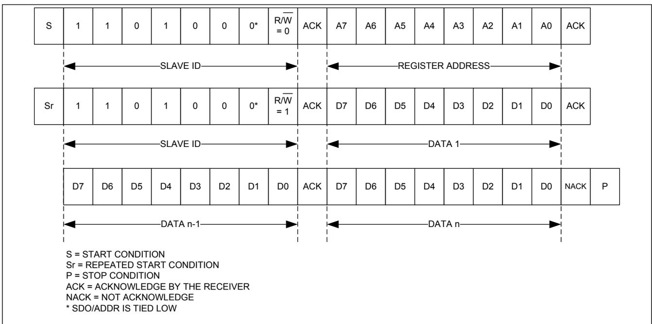
Figure 28. I<sup>2</sup>C Multibyte Read Transaction
