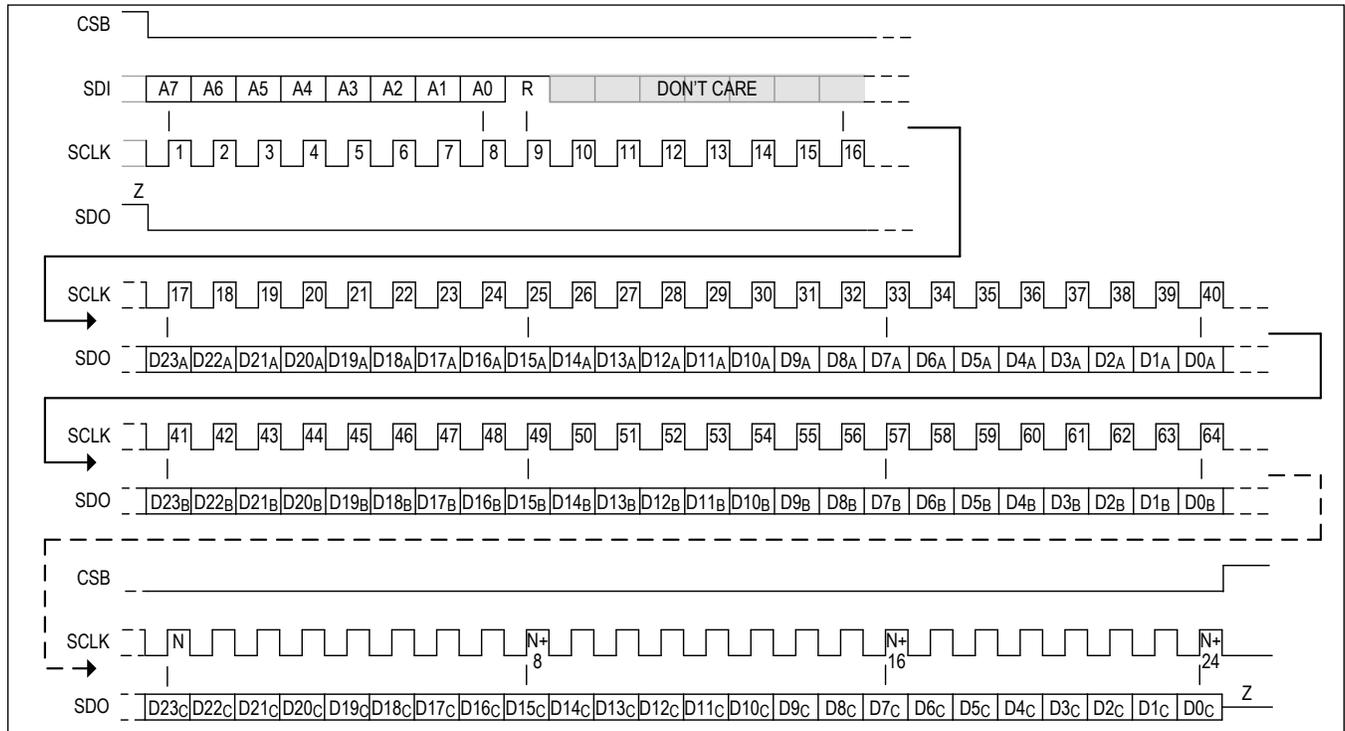
Figure 21. SPI FIFO Burst Mode Read Transaction
