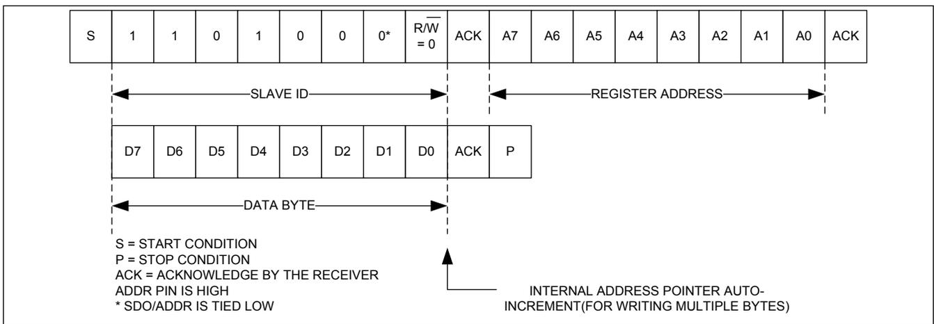
Figure 25. I<sup>2</sup>C Single-Byte Write Transaction
