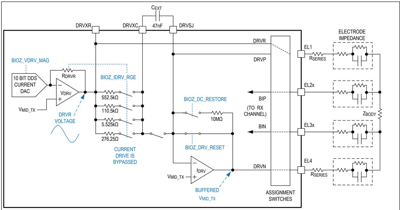
Figure 8. Bioimpedance Stimulus Generator — Sine-Wave Voltage Mode
