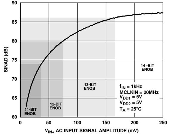
Figure 25. SINAD vs.  $V_{IN+}$  AC Input Signal Amplitude
