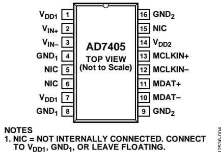
Figure 4. Pin Configuration
