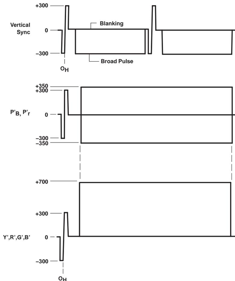
**Figure 14. SMPTE 274M Analog Interface Horizontal Timing Details†**
