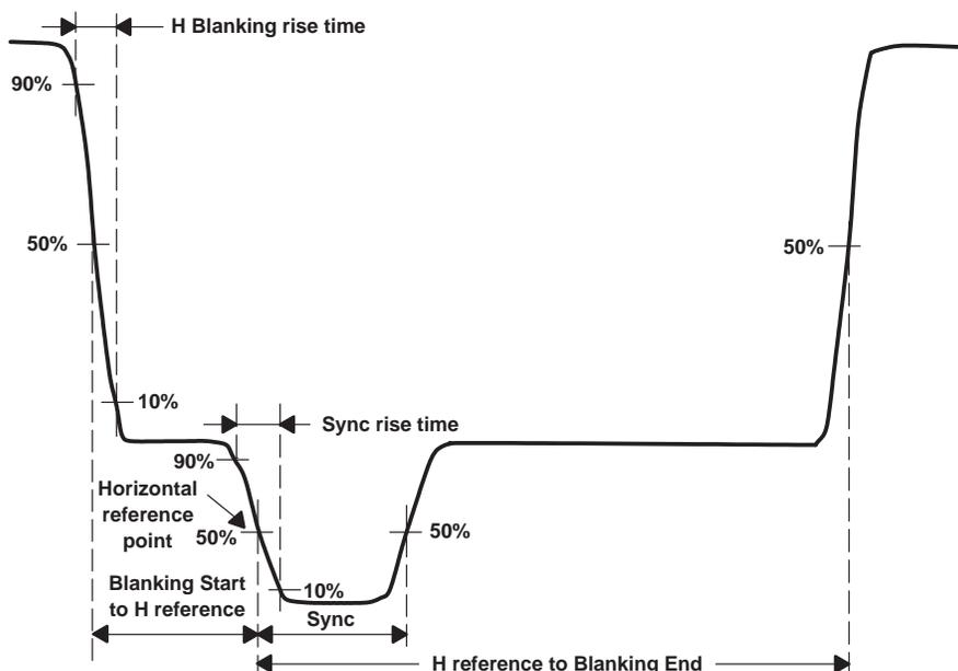
**Figure 12. SMPTE 253M Line Waveform (green channel)**
