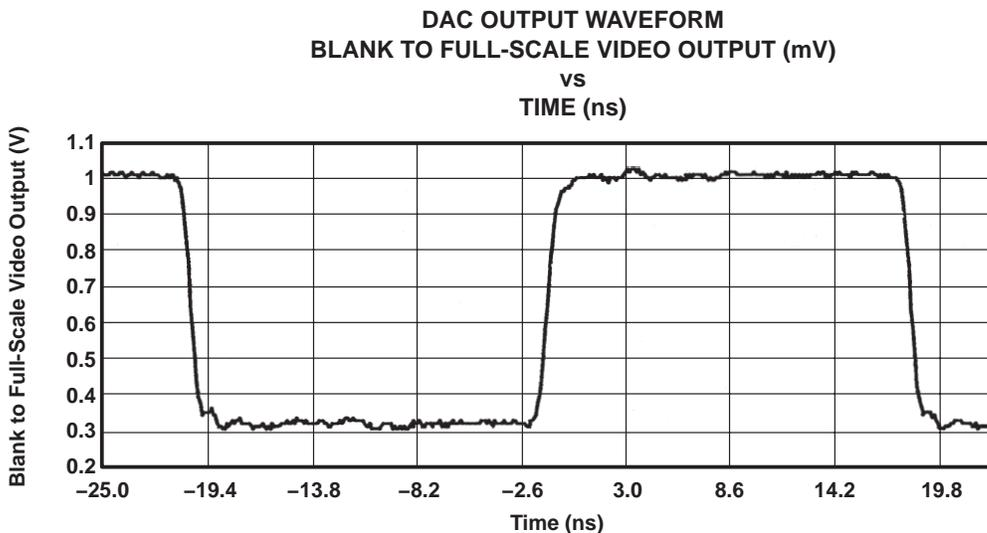
Figure 10. DAC Output Waveform (rise/fall and settling times)
