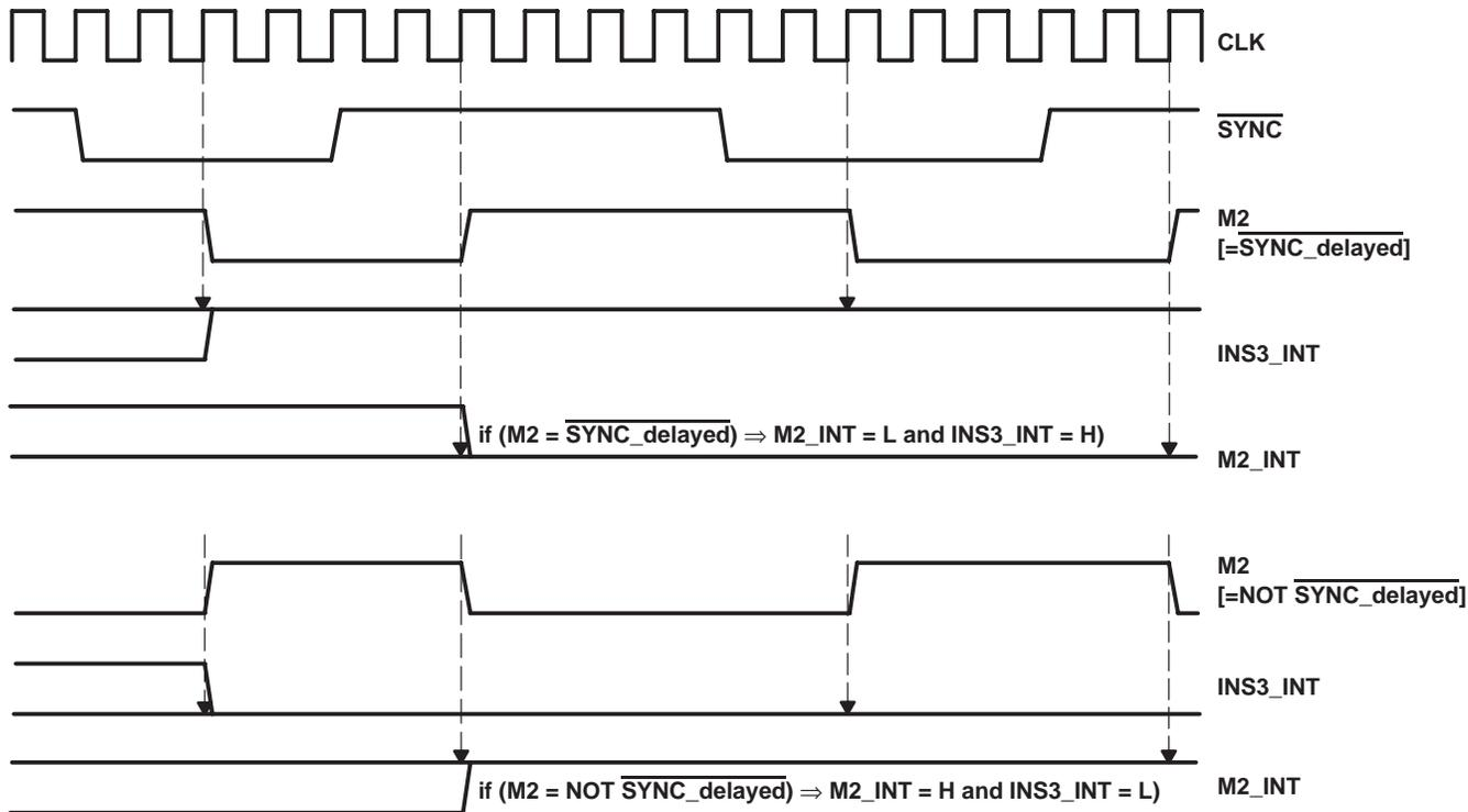
**Figure 2. Generating INS3\_INT and M2\_INT from M2**
