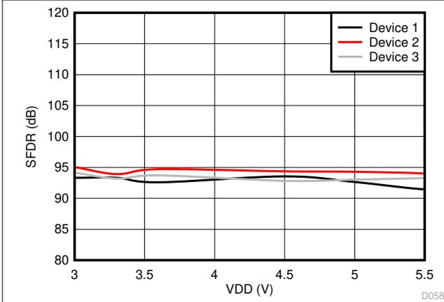
**Figure 6-32. Spurious-Free Dynamic Range vs Supply Voltage**
