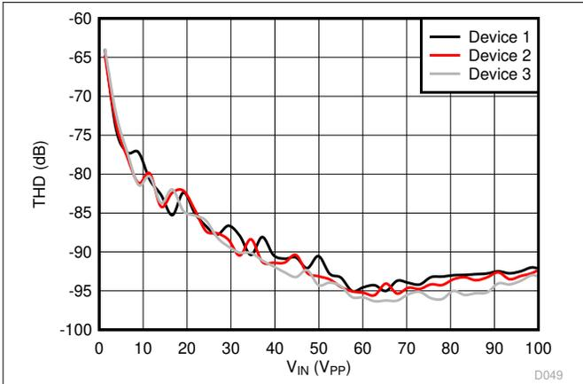
**Figure 6-24. Total Harmonic Distortion vs Input Signal Amplitude**
