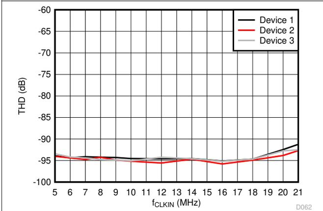
**Figure 6-26. Total Harmonic Distortion vs Input Clock Frequency**
