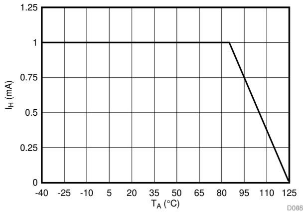
Figure 6-42. I<sub>H</sub> Derating vs Ambient Temperature
