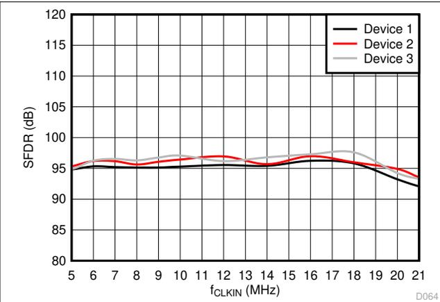
**Figure 6-31. Spurious-Free Dynamic Range vs Input Clock Frequency**
