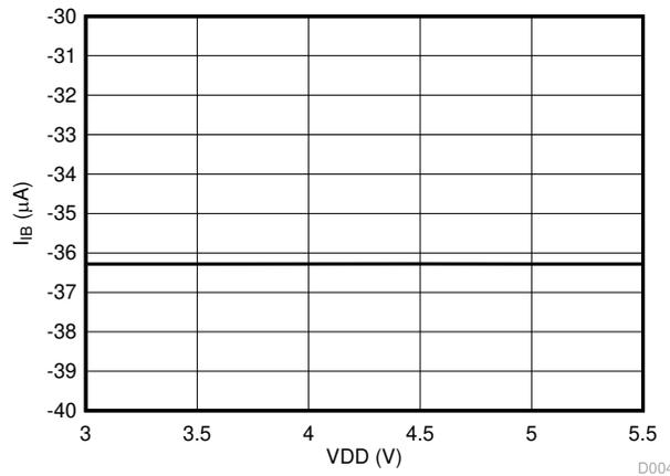
Figure 6-7. Input Bias Current vs Supply Voltage
