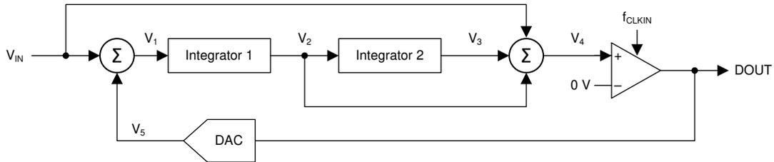
Figure 7-2. Block Diagram of a Second-Order Modulator
