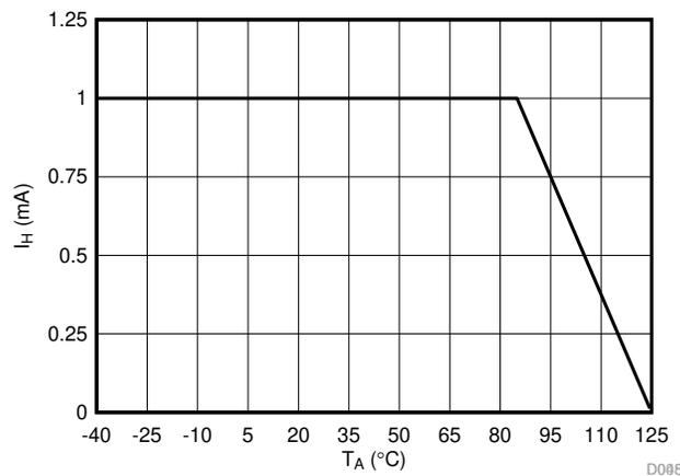
**Figure 7-6. Derating of  $I_H$  at Ambient Temperatures >85°C**
