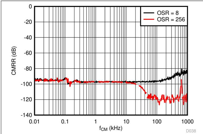
**Figure 6-36. Common-Mode Rejection Ratio vs Input Signal Frequency**
