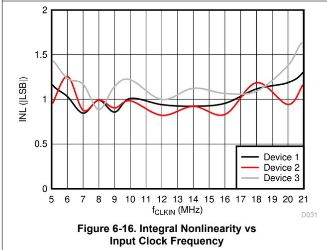
**Figure 6-16. Integral Nonlinearity vs Input Clock Frequency**
