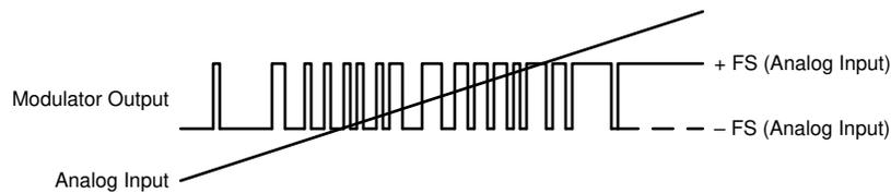
**Figure 7-4. AMC3306M05 Modulator Output vs Analog Input**
