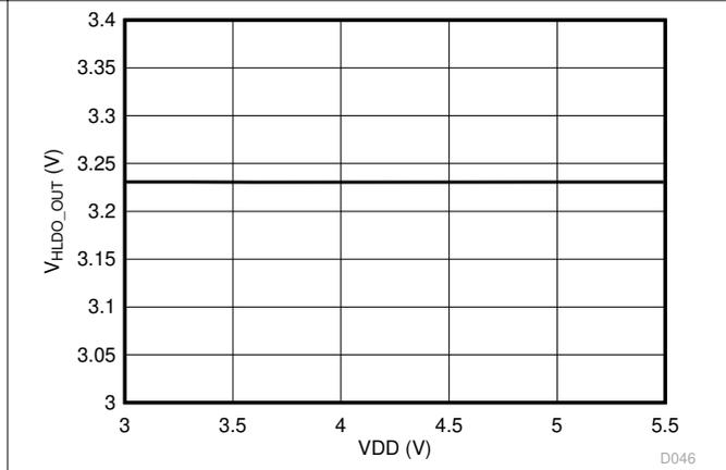
**Figure 6-41. High-Side LDO Output Voltage vs Supply Voltage**
