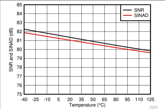
Figure 6-23. Signal-to-Noise Ratio and Signal-to-Noise + Distortion vs Temperature
