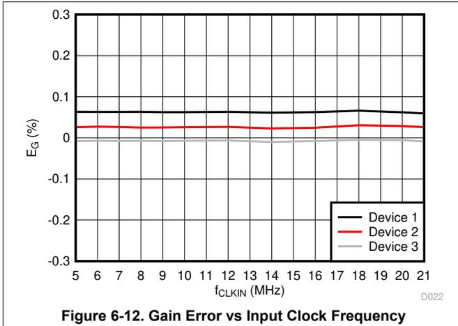
**Figure 6-12. Gain Error vs Input Clock Frequency**
