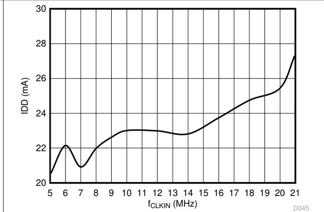
**Figure 6-39. Supply Current vs Input Clock Frequency**
