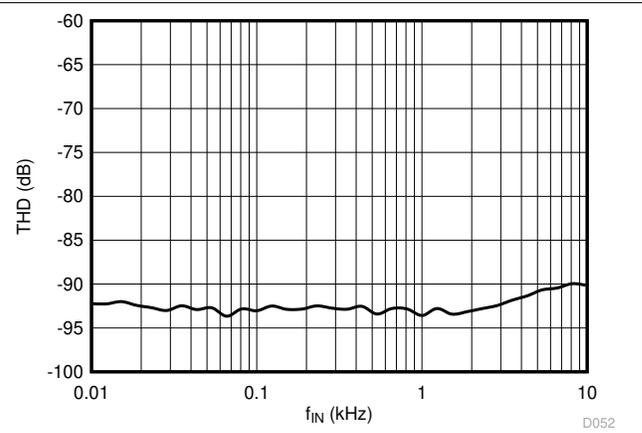
**Figure 6-25. Total Harmonic Distortion vs Input Signal Frequency**
