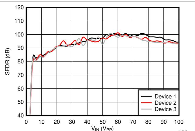
**Figure 6-29. Spurious-Free Dynamic Range vs Input Signal Amplitude**
