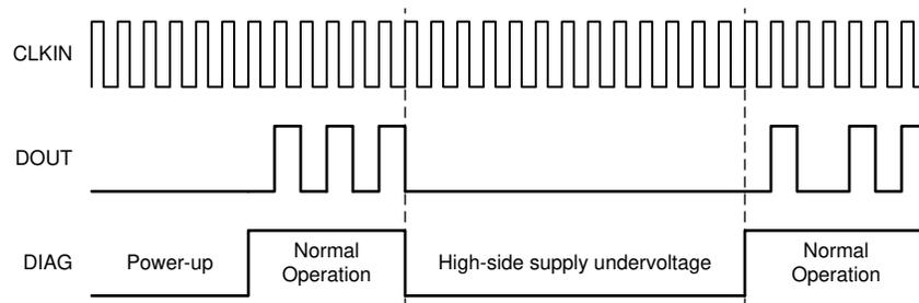
**Figure 7-7. DIAG and Output Under Different Operating Conditions**
