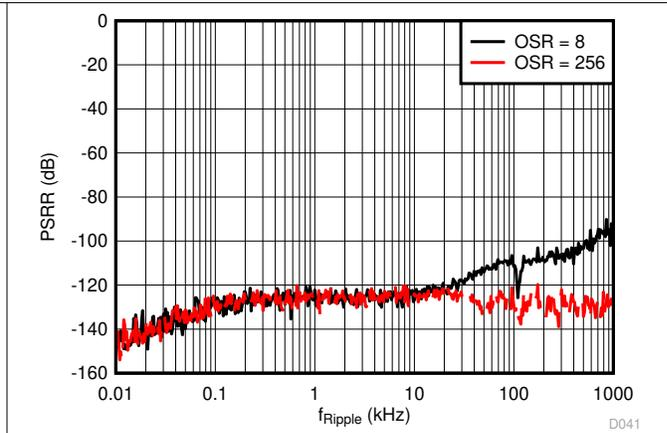
**Figure 6-37. Power-Supply Rejection Ratio vs Ripple Frequency**
