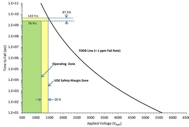
$T_A$  up to 150°C, stress-voltage frequency = 60 Hz, isolation working voltage = 1200  $V_{RMS}$ , operating lifetime = 76 years
