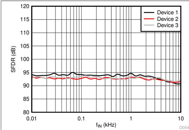
**Figure 6-30. Spurious-Free Dynamic Range vs Input Signal Frequency**
