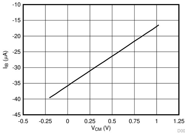
Figure 6-6. Input Bias Current vs Common-Mode Input Voltage
