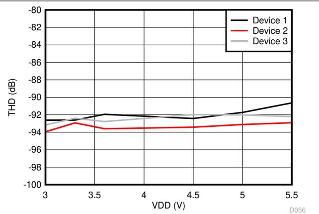
**Figure 6-27. Total Harmonic Distortion vs Supply Voltage**
