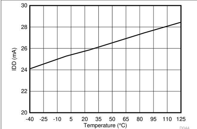
**Figure 6-40. Supply Current vs Temperature**
