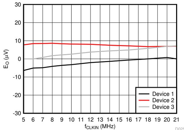
Figure 6-9. Offset Error vs Input Clock Frequency
