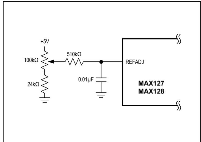
Figure 12. Reference-Adjust Circuit
