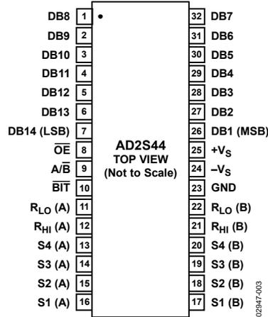
Figure 2. Pin Configuration
