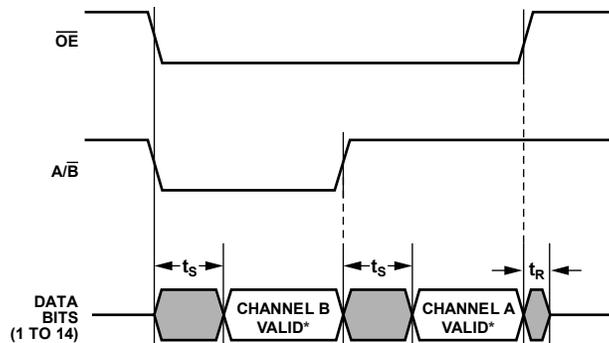
\*CONVERTER DATA OUTPUT IS INHIBITED FROM UPDATES DURING CHANNEL VALID.
