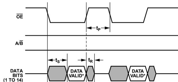
\*CONVERTER DATA OUTPUT IS INHIBITED FROM UPDATES DURING CHANNEL VALID.
